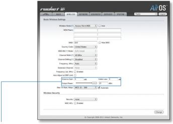
Since Ubiquiti Networks equipment can be paired with a variety of antennas and cables, the *Antenna Gain*, *Cable Loss*, and *Output Power* fields are provided to the professional installer to assist in meeting regulatory requirements.
