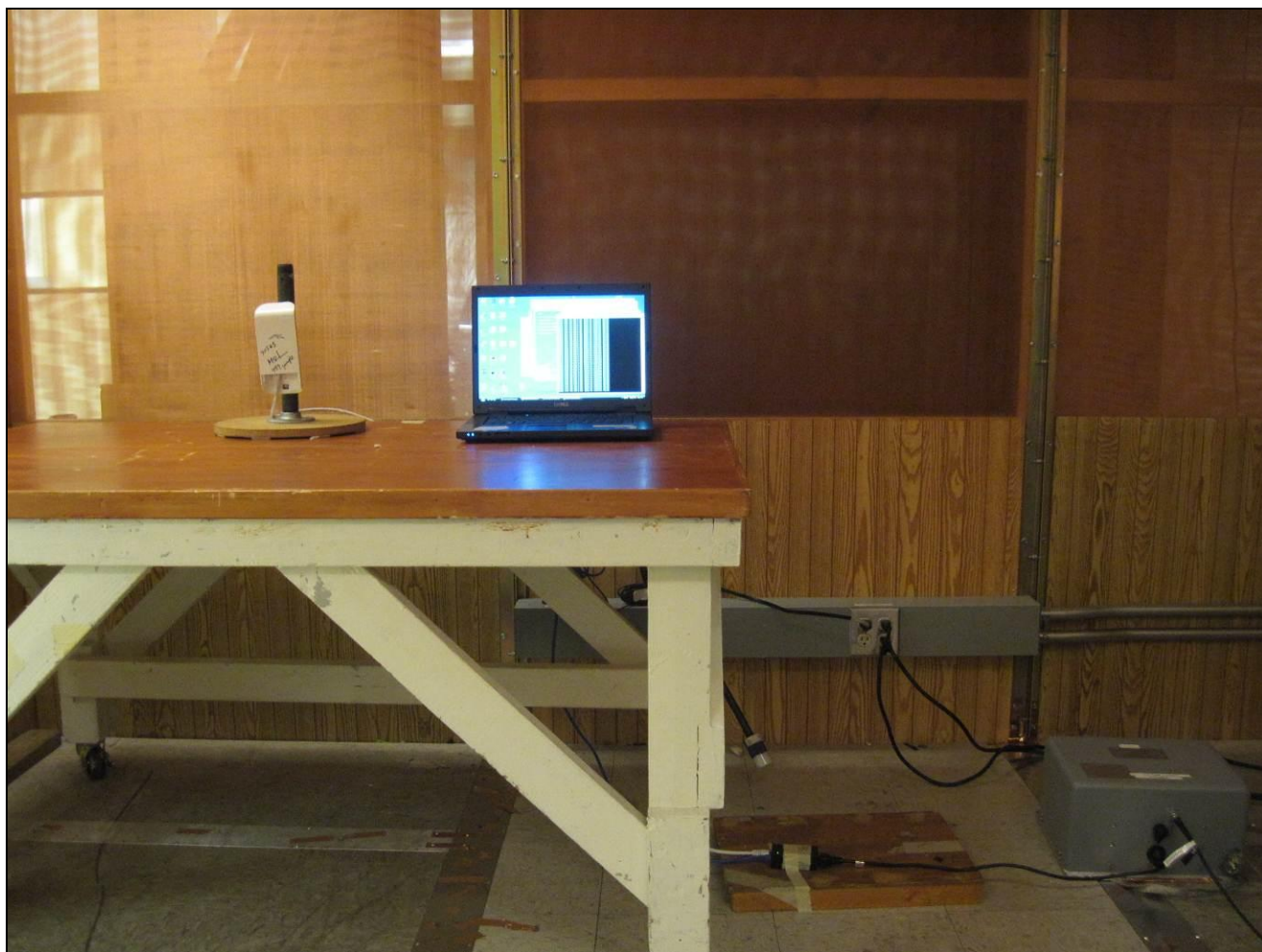
Photograph 1. Conducted Emissions, Test Setup
