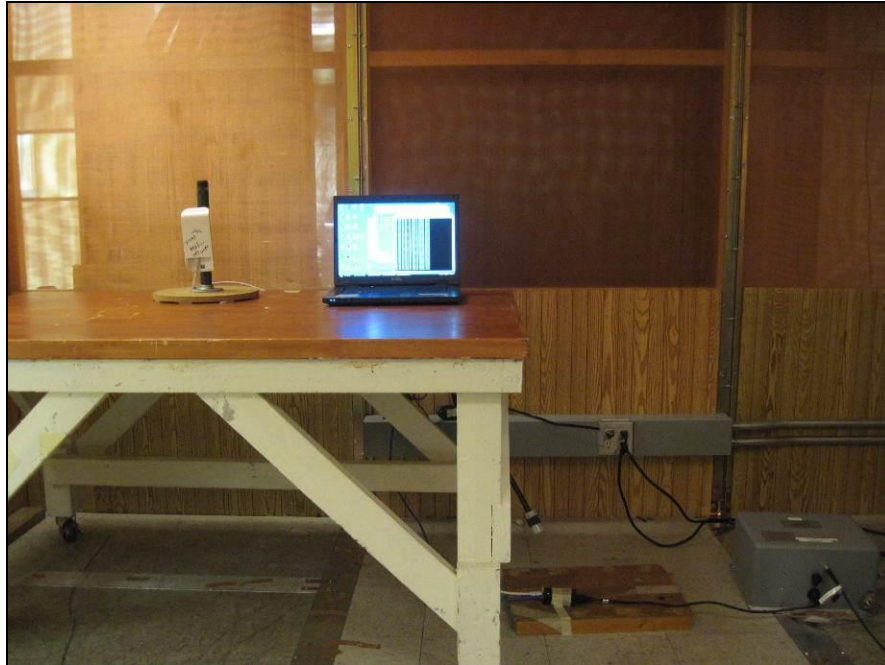
Photograph 5. Conducted Emissions, 15.207(a), Test Setup
