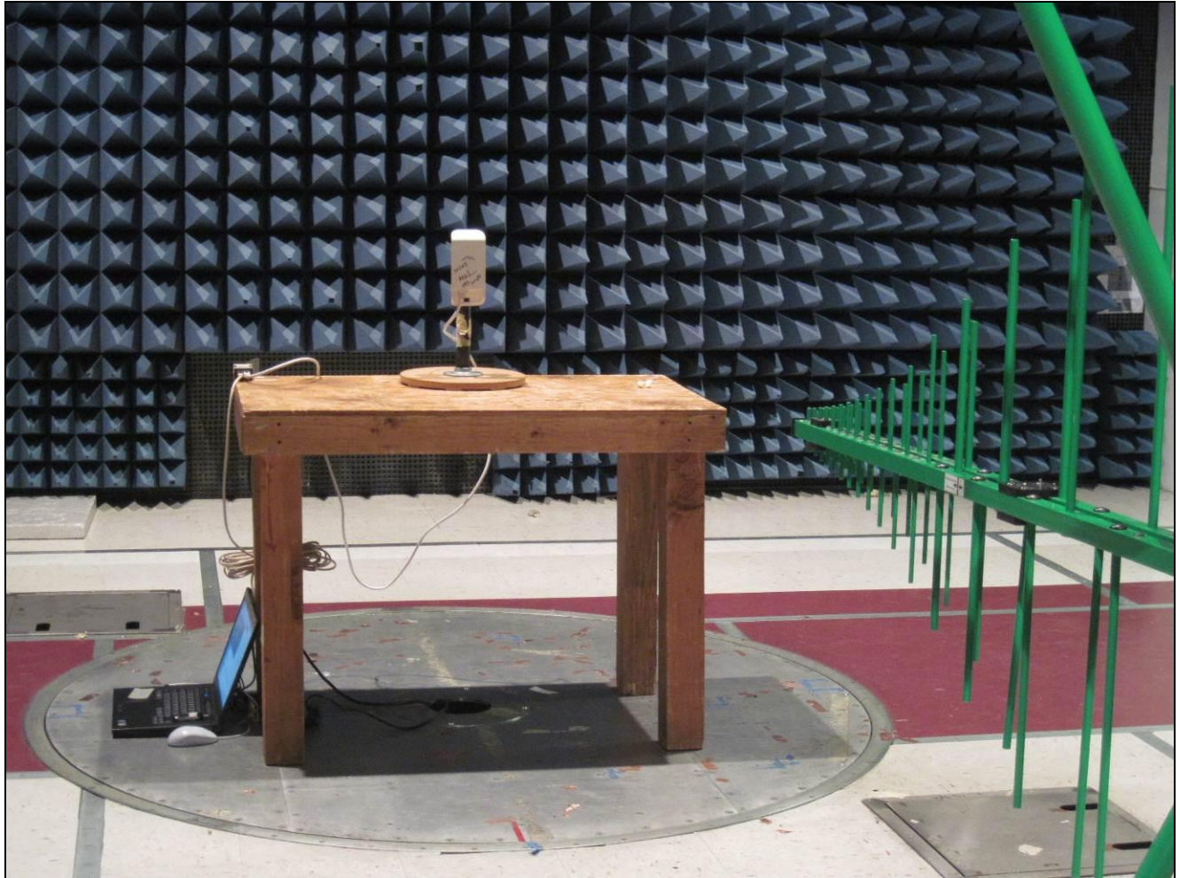
Photograph 3. Radiated Emission, Test Setup, CETUS
