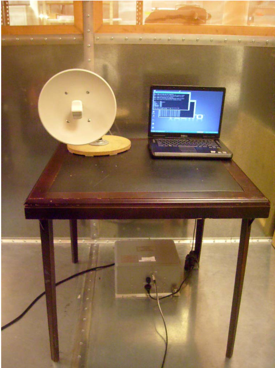
Photograph 1. Conducted Emissions, Test Setup
