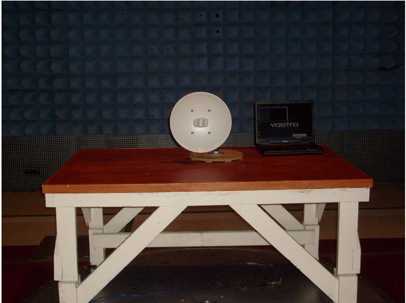
Photograph 3. Radiated Emission, Test Setup
