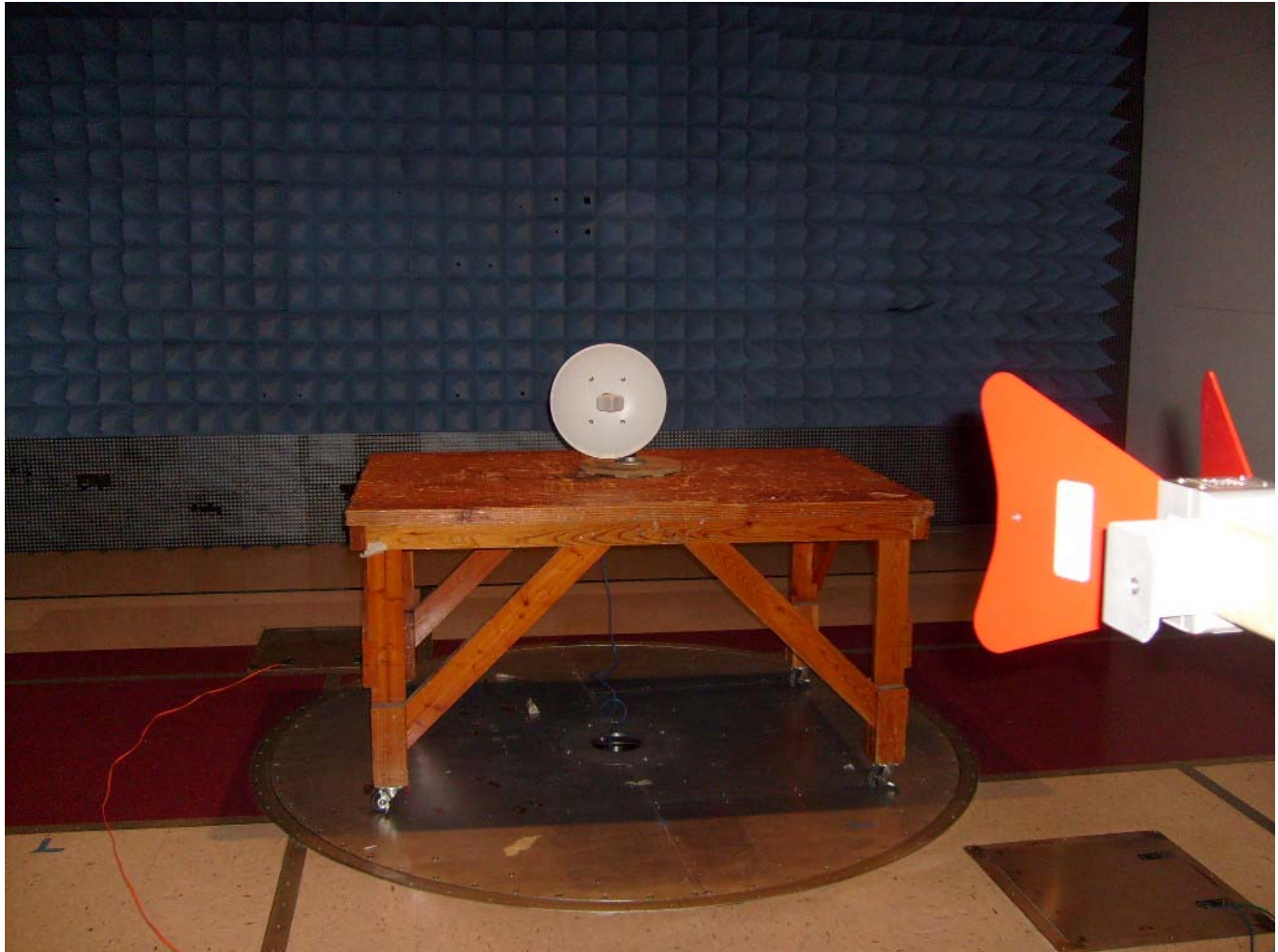
Photograph 6. Radiated Spurious, Test Setup (Dish Antenna)
