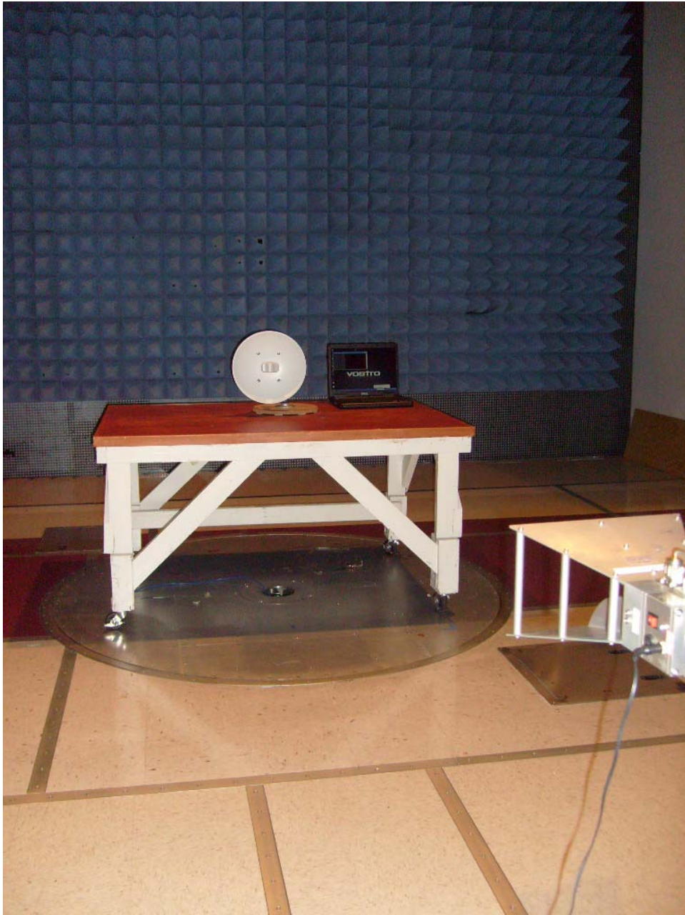
Photograph 4. Radiated Emission, above 1GHz Test Setup
