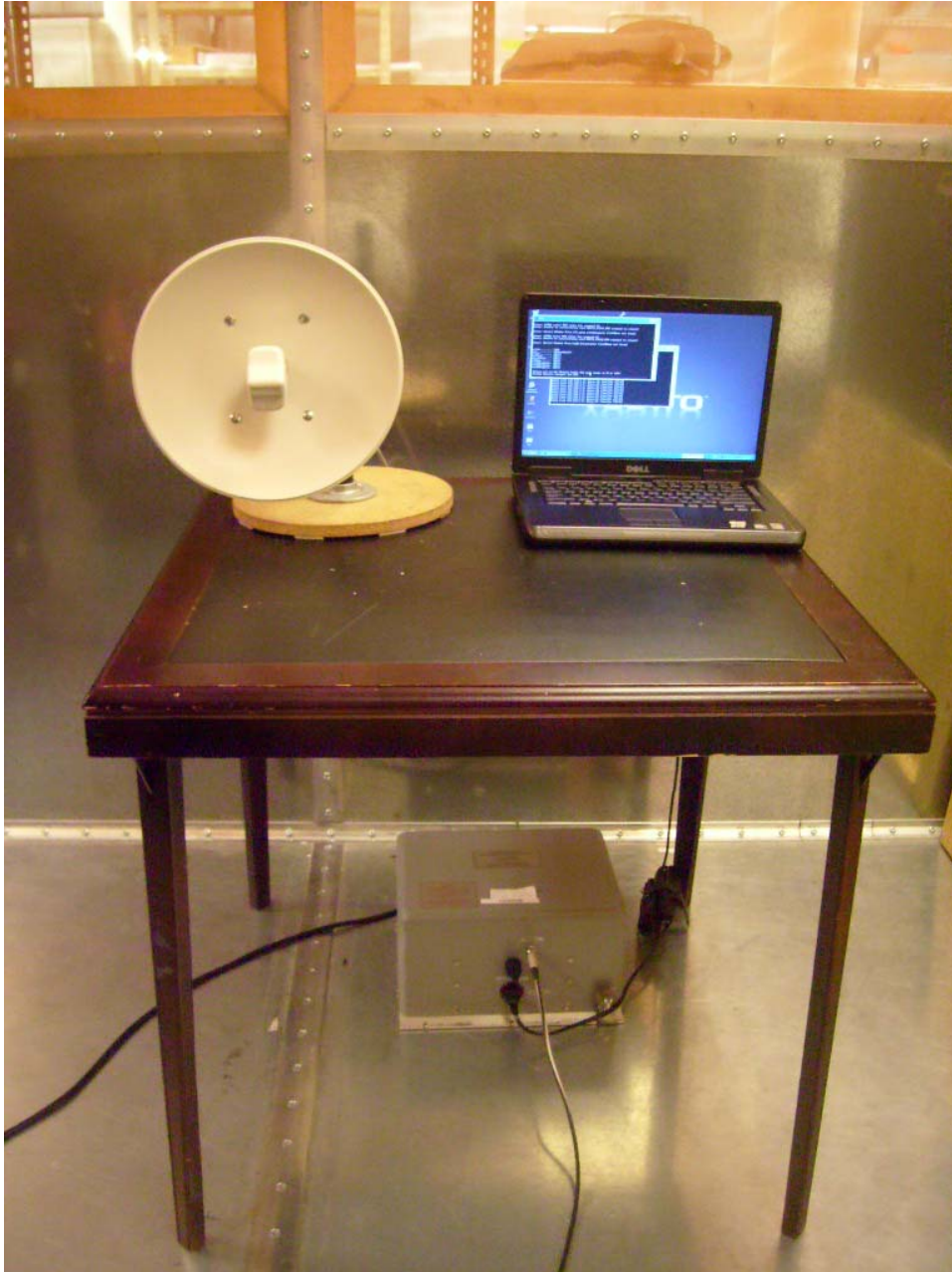
Photograph 5. Conducted Emissions, 15.207, Test Setup
