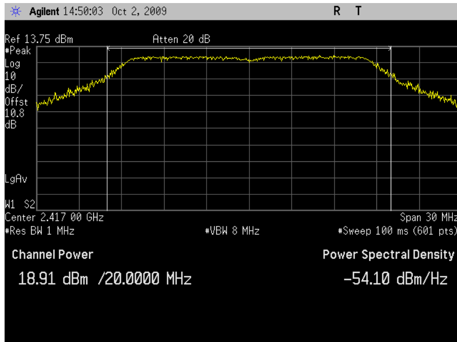
Plot 17. Peak Output Power, HT20 Channel 2 - Dish Antenna
