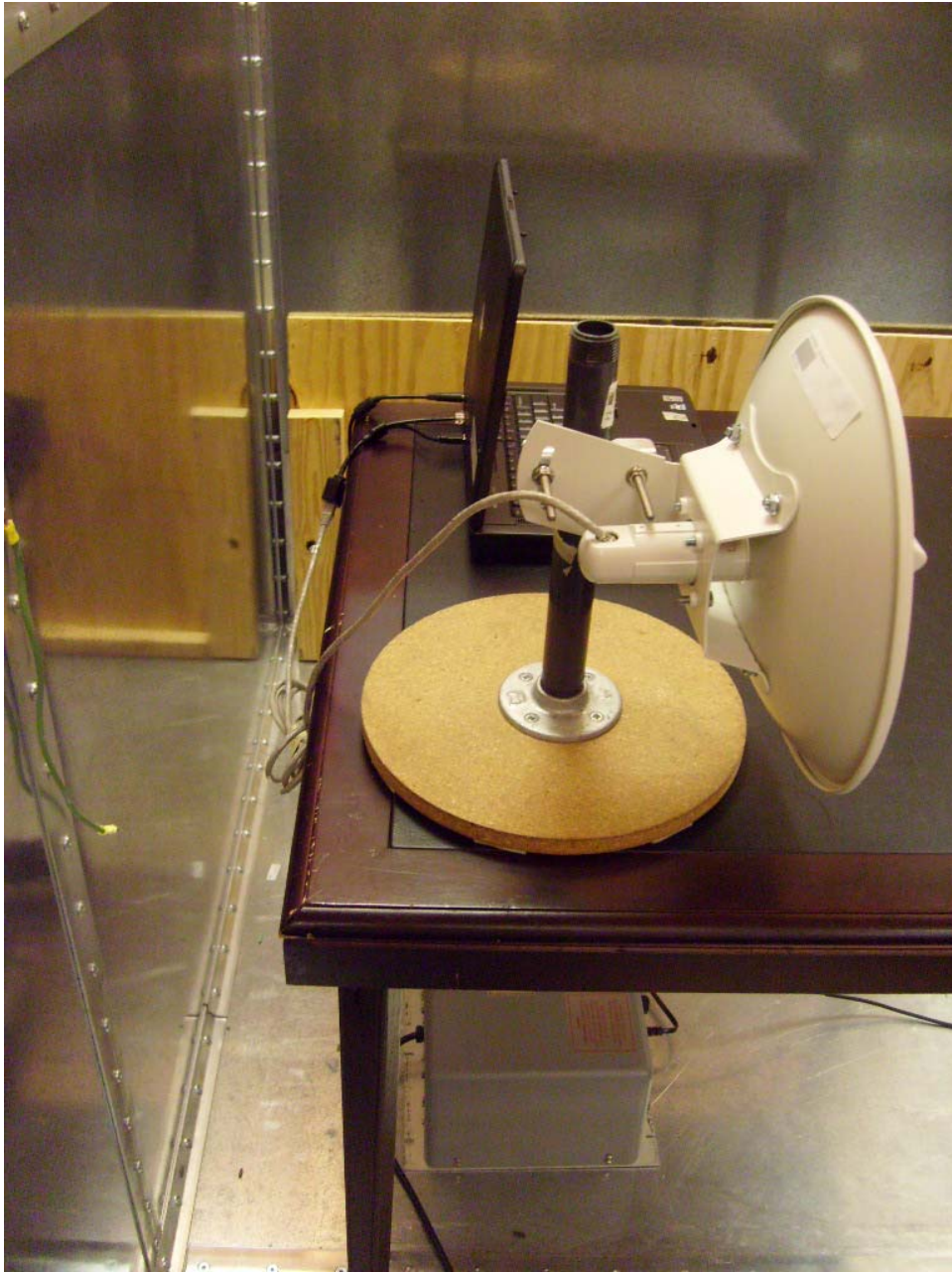
Photograph 2. Conducted Emissions, Test Setup
