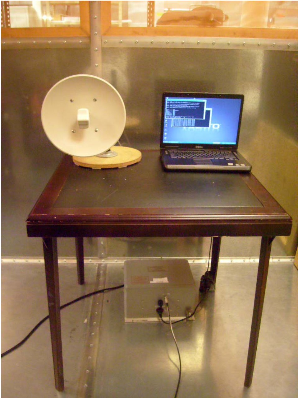
Photograph 1. Conducted Emissions, Test Setup
