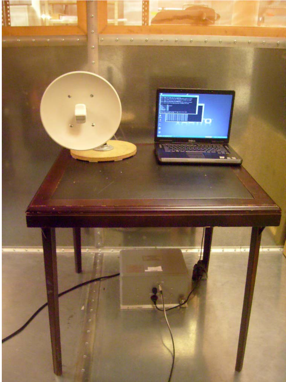
Photograph 5. Conducted Emissions, 15.207, Test Setup
