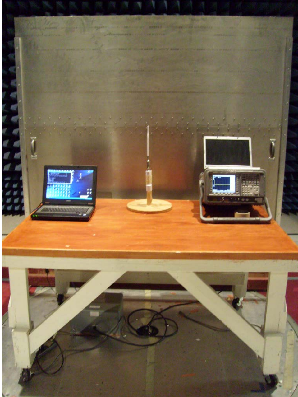
Photograph 1. Conducted Emissions, Test Setup
