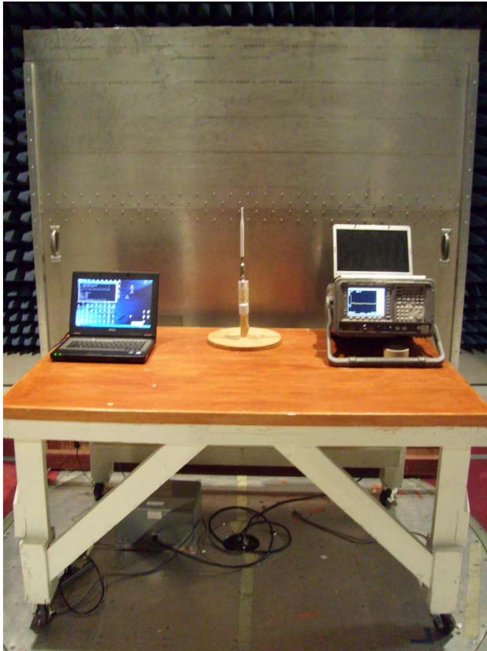
Photograph 4. Conducted Emissions, 15.207, Test Setup
