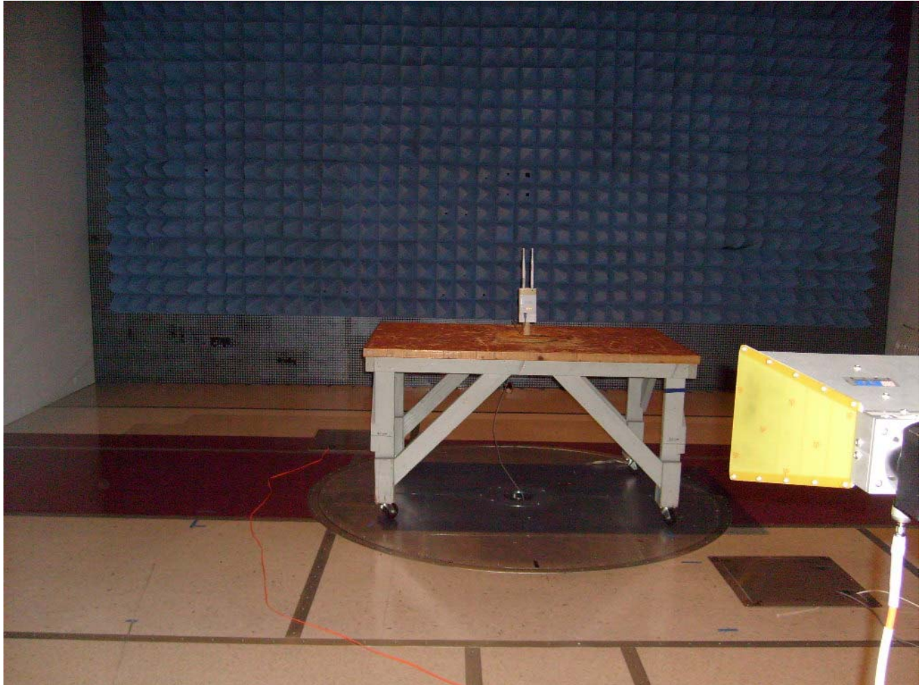
Photograph 6. Test Equipment and setup for various Radiated Measurements – 6dBi Omni Antenna
