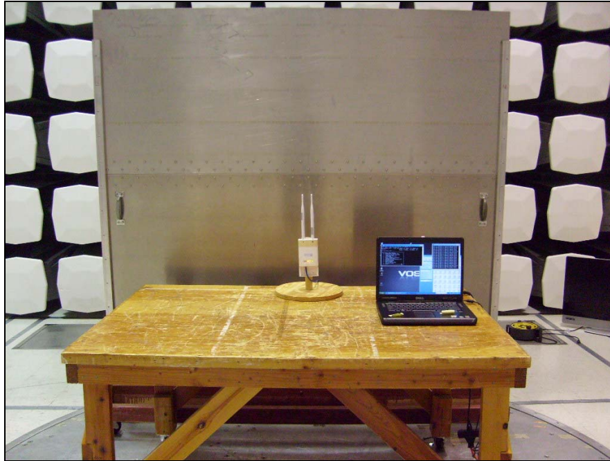
Photograph 5. Conducted Emissions Test Setup
