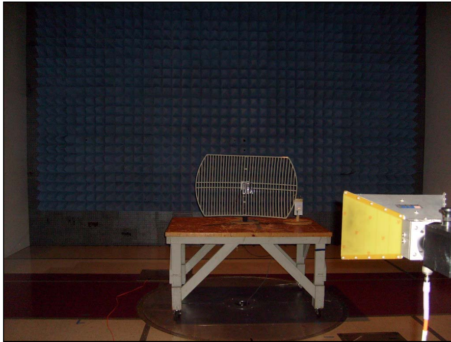
Photograph 9. Test Equipment and setup for various Radiated Measurements – 25dBi Grid Antenna
