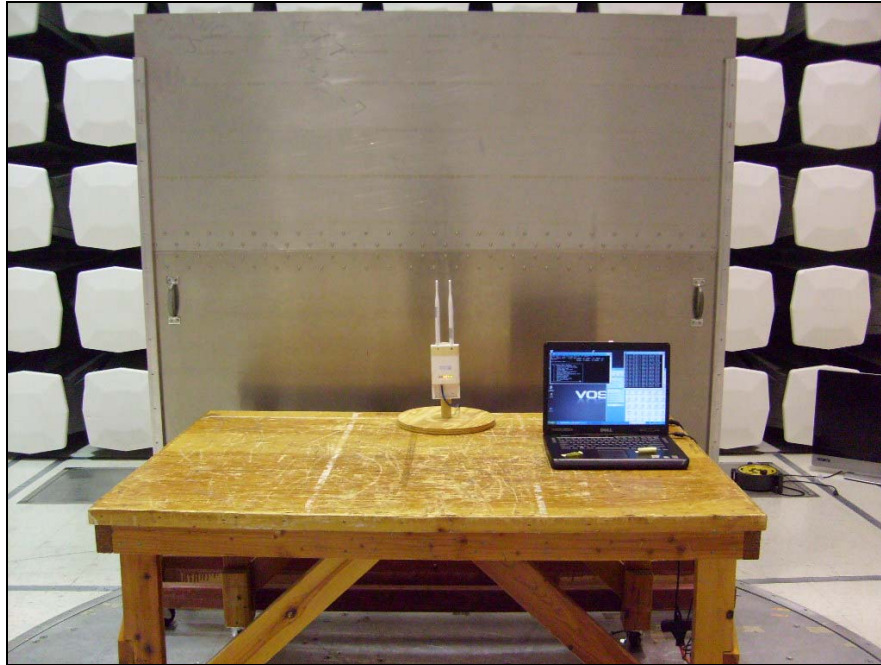
Photograph 2. Conducted Emissions Test Setup
