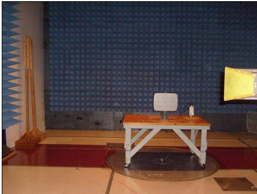
Photograph 8. Test Equipment and setup for Various Radiated Measurements – 18dBi Panel Antenna
