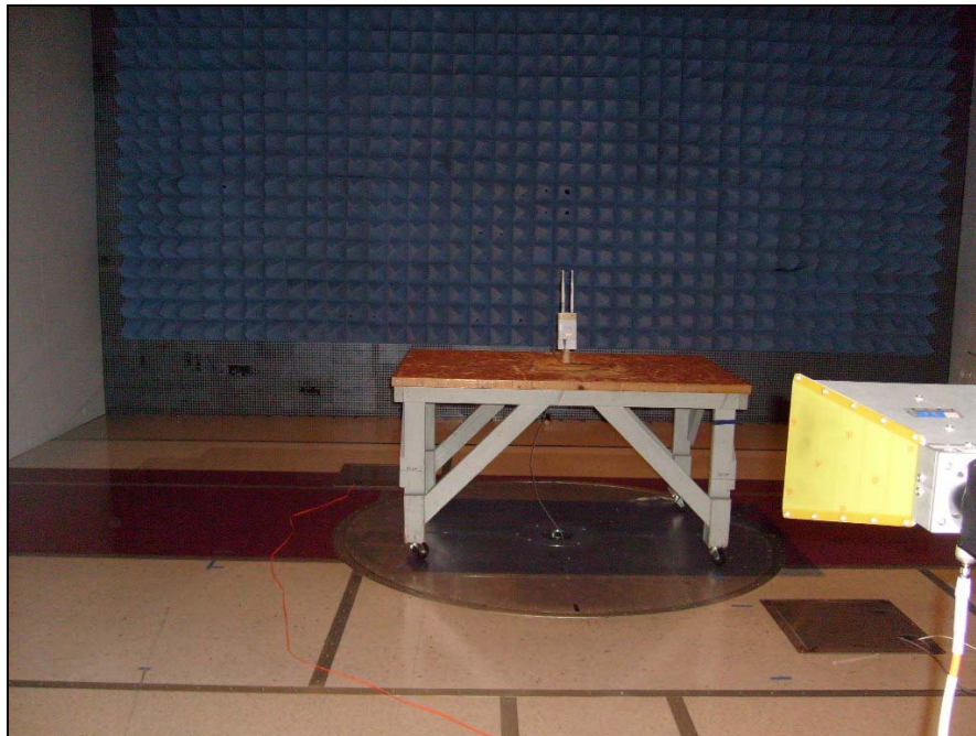
Photograph 10. Test Equipment and setup for various Radiated Measurements – Combined Omni Antennas
