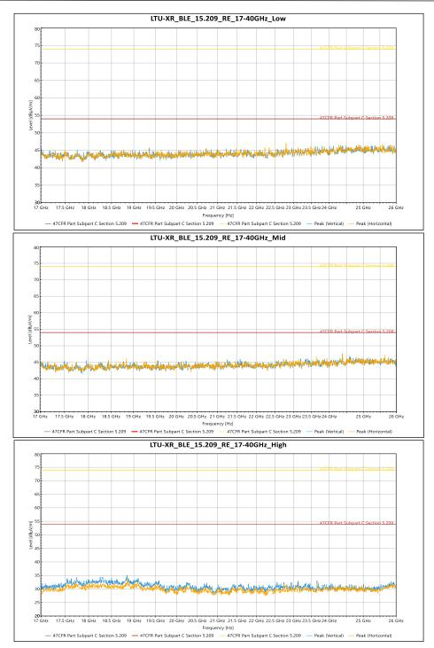
Vertical: No significant emissions were observed in this frequency range.
