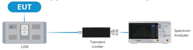
**Figure 1: Conducted Emissions Test**
