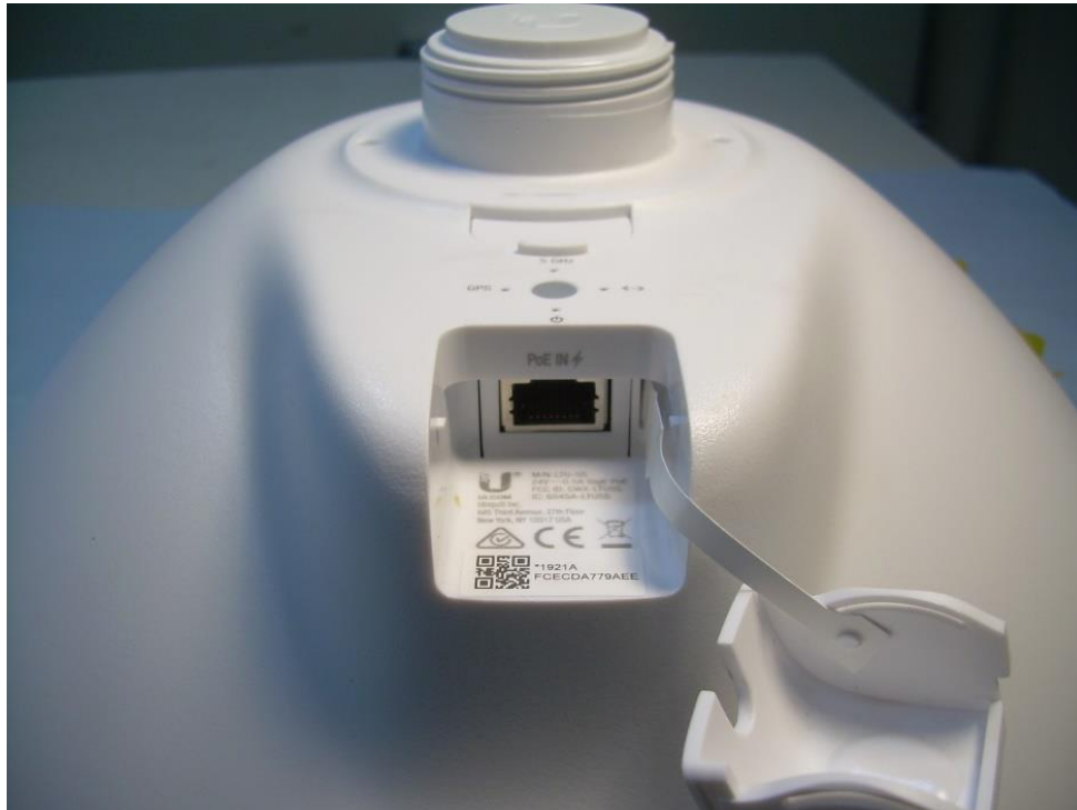
Photograph 3 – View of Data/Power Port
