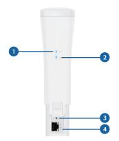
**LAN LED** The LED will light steady blue when an active Ethernet connection is made to the Ethernet port and flash when there is activity.
