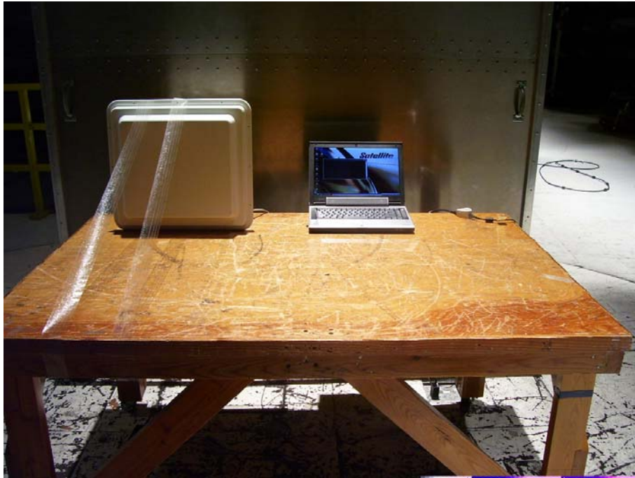
Photograph 2. Conducted Emissions Test Setup, Front View
