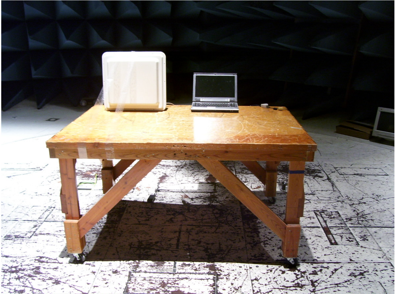
Photograph 4. Radiated Emission Limits Test Setup
