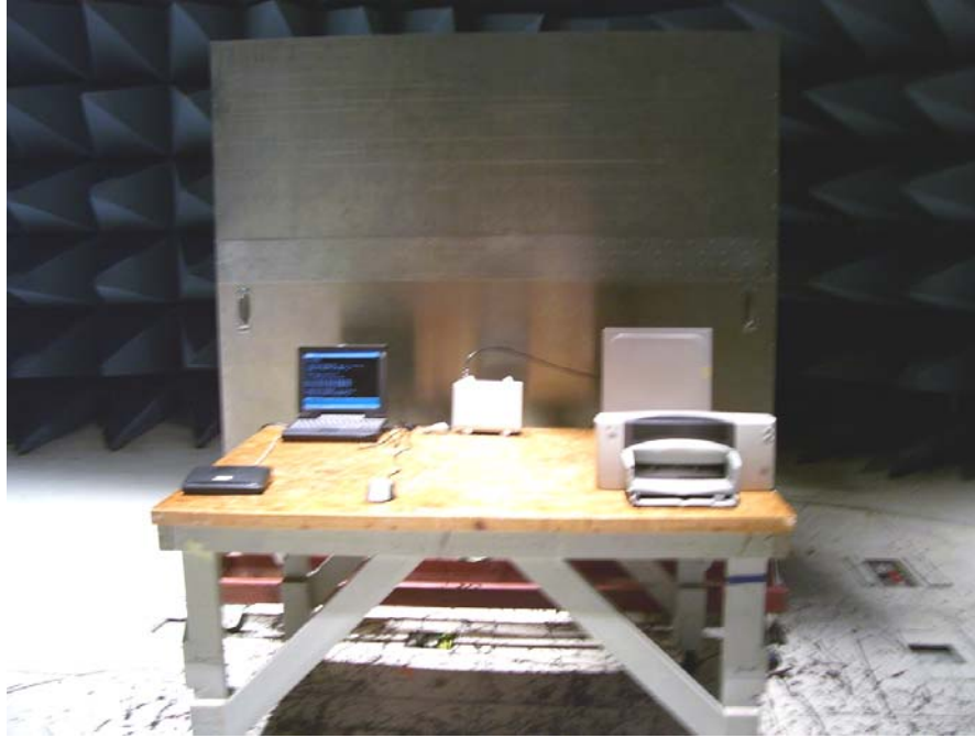
Photograph 2. Conducted Emissions Test Setup, Front
