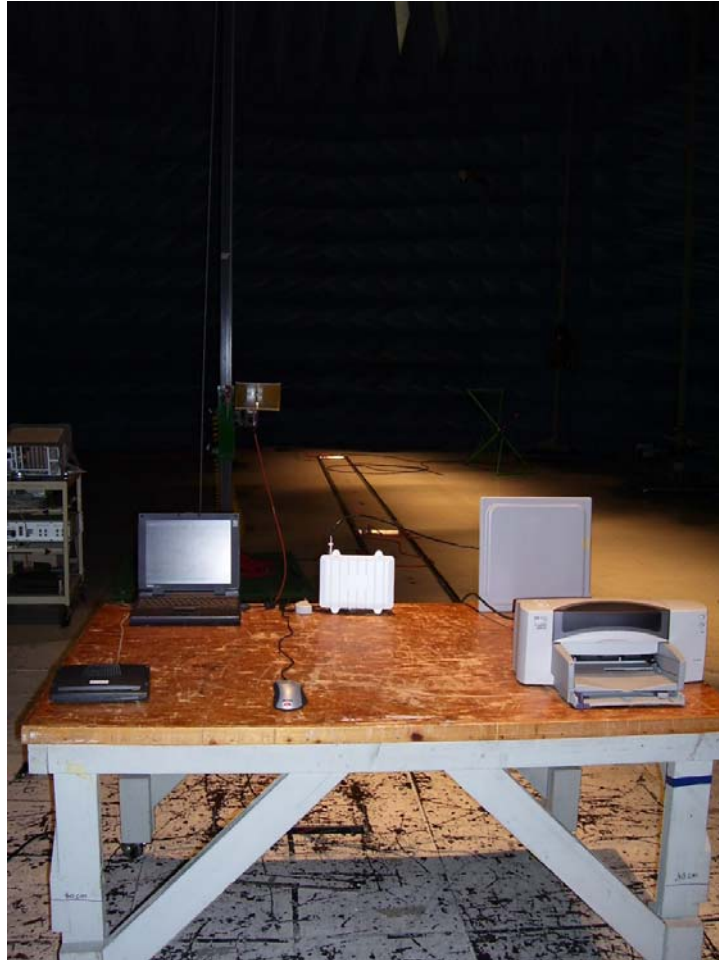
Photograph 4. Radiated Emission Limits Test Setup
