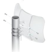
5. You have  $\pm 15^\circ$  of elevation adjustment available. Aim the LiteBeam toward the other end of the wireless link.
