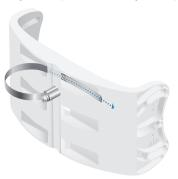
To mount the Mounting Bracket, wrap each Metal Strap around the pole. Use a 7 mm socket wrench or screwdriver to turn the screw clockwise and securely fasten the strap to the pole.
