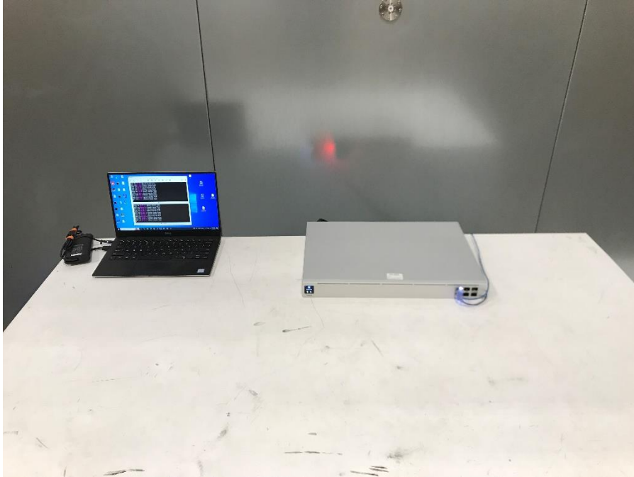
Photograph 1: Front View Test Set Up Conducted Emissions
