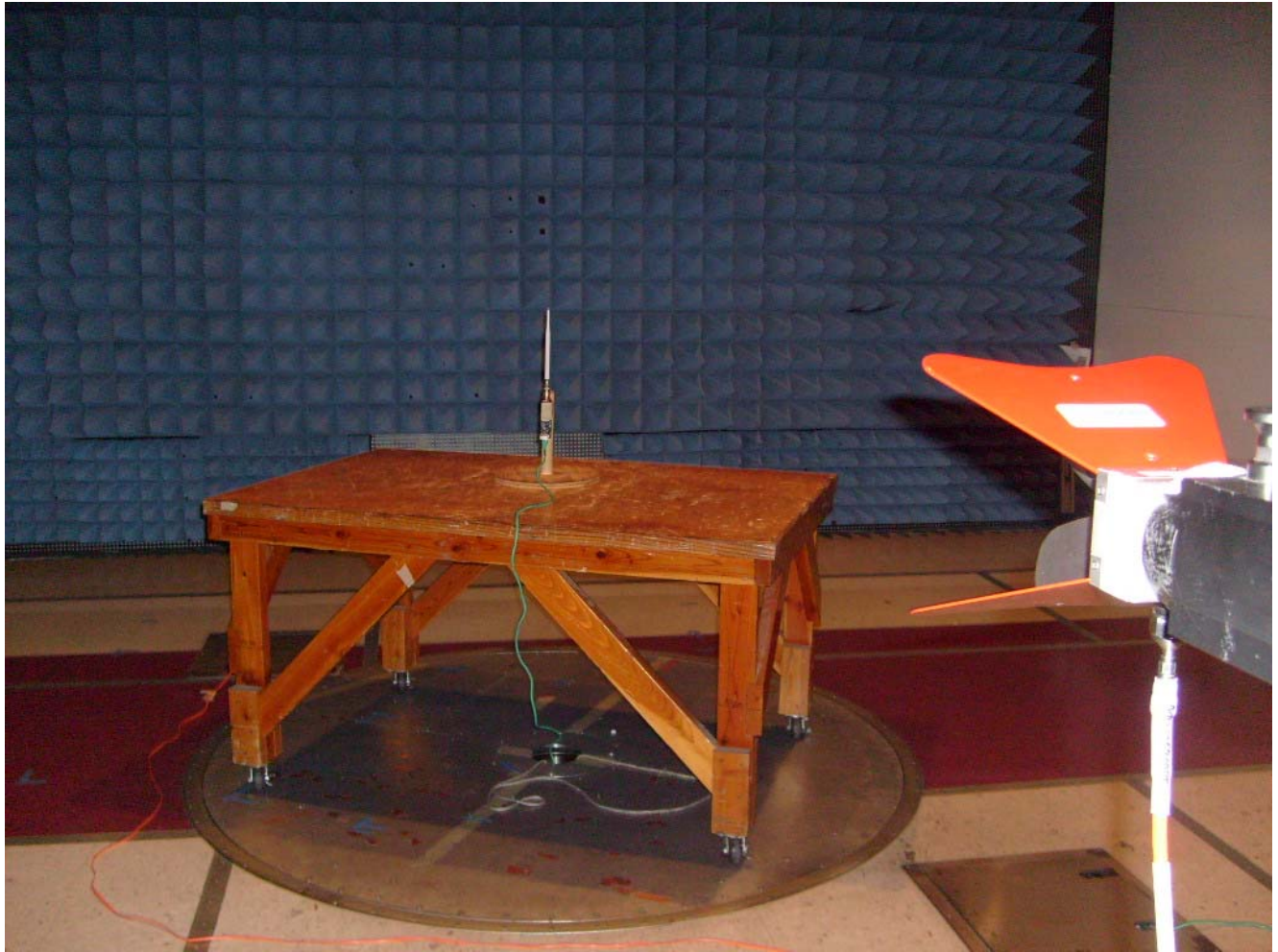
Photograph 7. Radiated Spurious Emission, 3m Test Setup (6dBi Omni Antenna)
