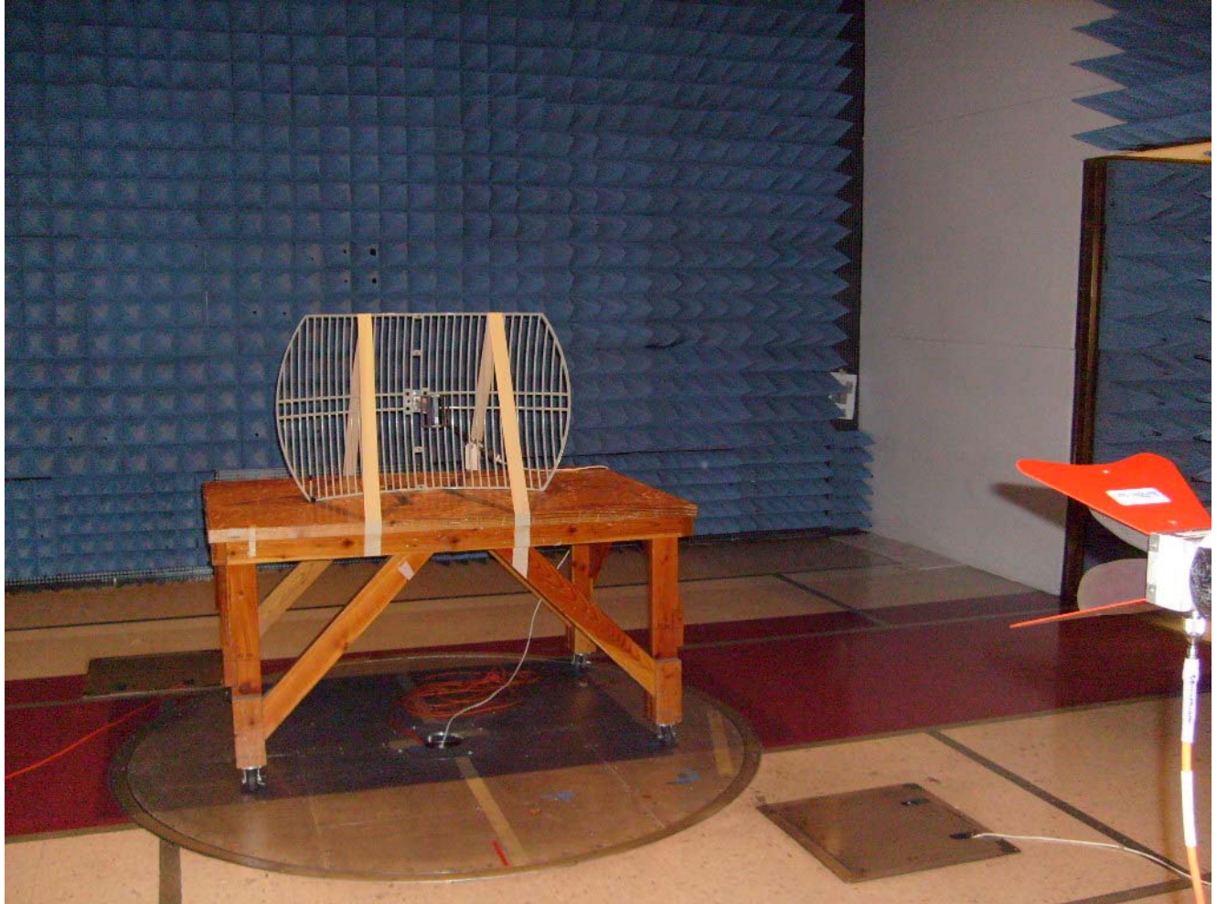
Photograph 8. Radiated Spurious Emission, Test Setup (24dBi Grid Antenna)
