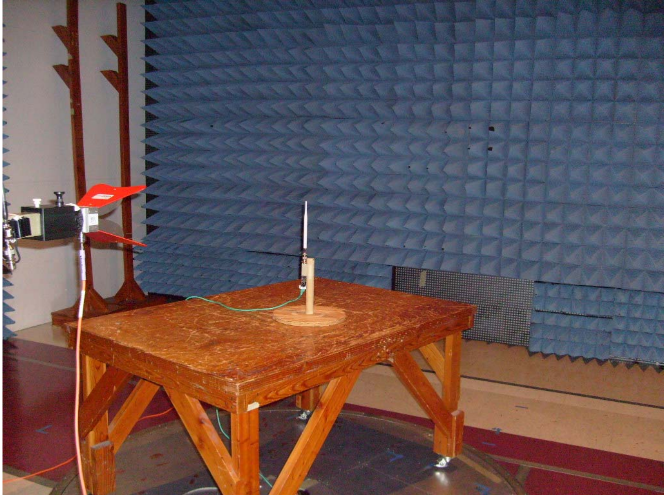
Photograph 6. Radiated Spurious Emission, 1m Test Setup (6dBi Omni Antenna)
