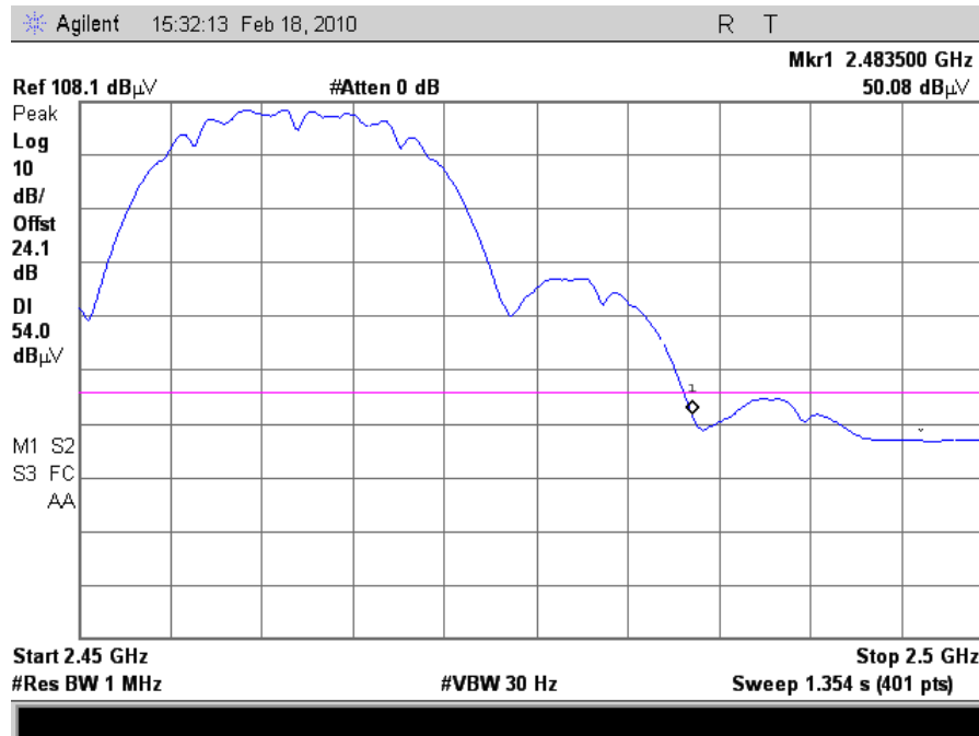
Plot 72. 802.11b Higher Band Edge, Channel 11, Average (6dBi Omni Antenna)
