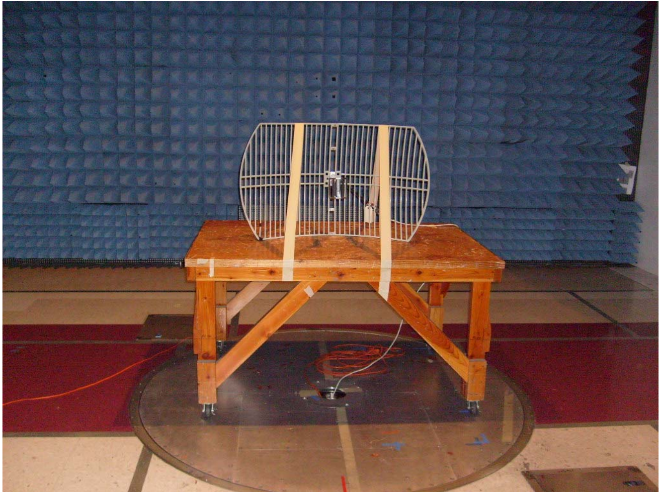
Photograph 9. Radiated Spurious Emission, Test Setup (24dBi Grid Antenna)
