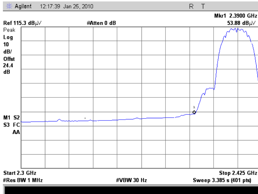
Plot 82. 802.11b Lower Band Edge, Channel 1, Average (24dBi Grid Antenna)
