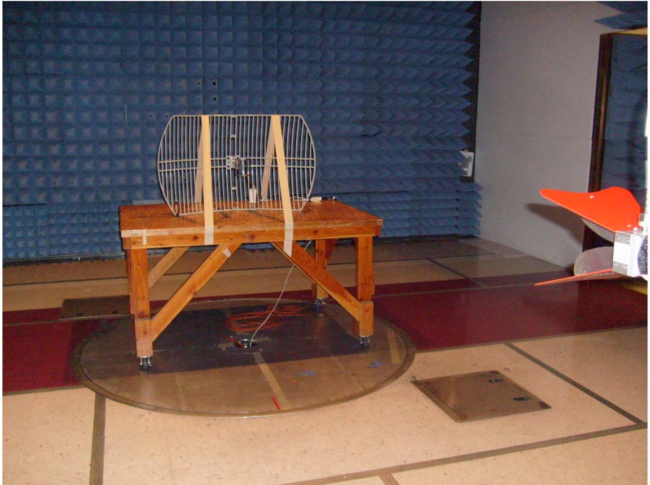
Photograph 4. Radiated Emission, above 1GHz Test Setup
