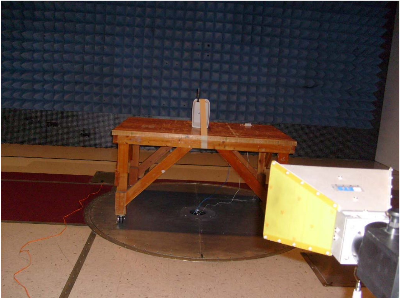
Photograph 4. Radiated Emission Test Setup 1GHz – 2GHz
