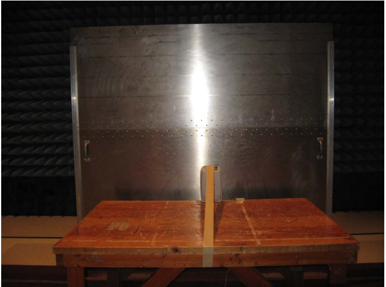
Photograph 2. Conducted Emissions Test Setup
