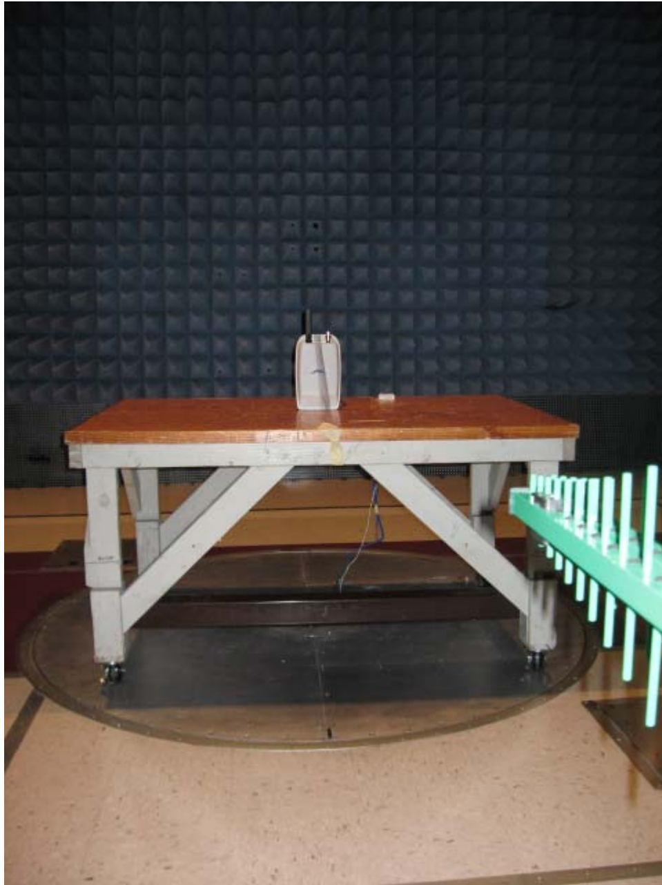
Photograph 3. Radiated Emission Test Setup 30 MHz - 1 GHz
