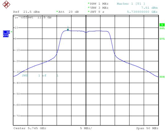
Modulation Standard: 802.11ac, VHT20 (6.5Mbps)
