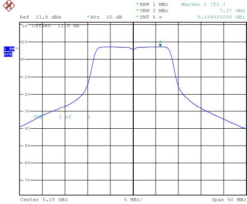
Modulation Standard: 802.11ac VHT20 (6.5Mbps)
