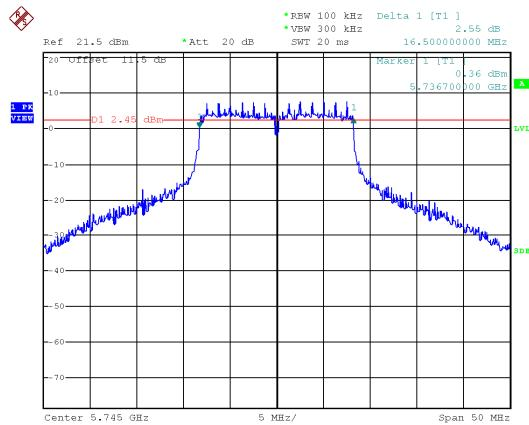
Modulation Standard: 802.11ac, VHT20 (6.5Mbps)
