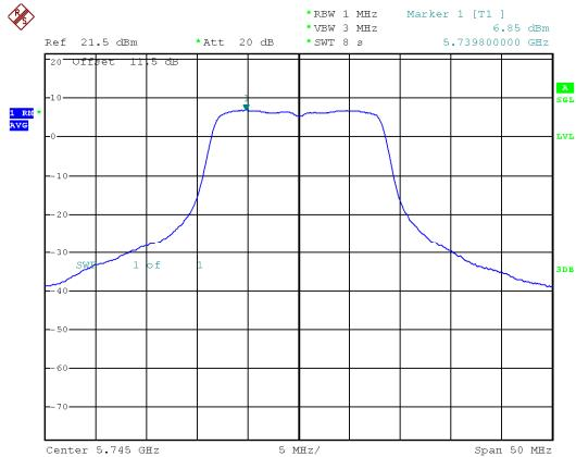
Modulation Standard: 802.11ac, VHT20 (6.5Mbps)
