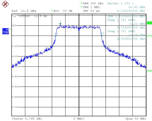
Modulation Standard: 802.11ac, VHT20 (6.5Mbps)
