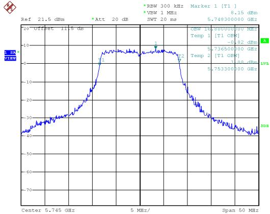
Modulation Standard: 802.11ac, VHT20 (6.5Mbps)
