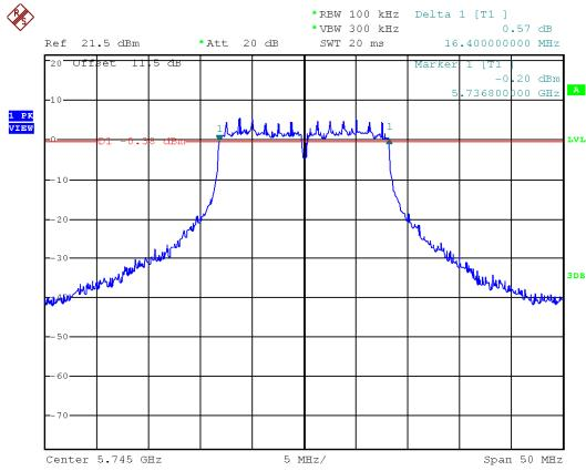
Modulation Standard: 802.11ac, VHT20 (6.5Mbps)
