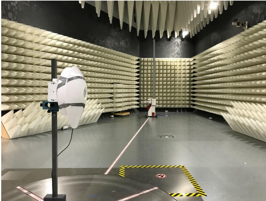
Photograph 1: View Test Set Up Radiated Emissions 30 – 1000 MHz
