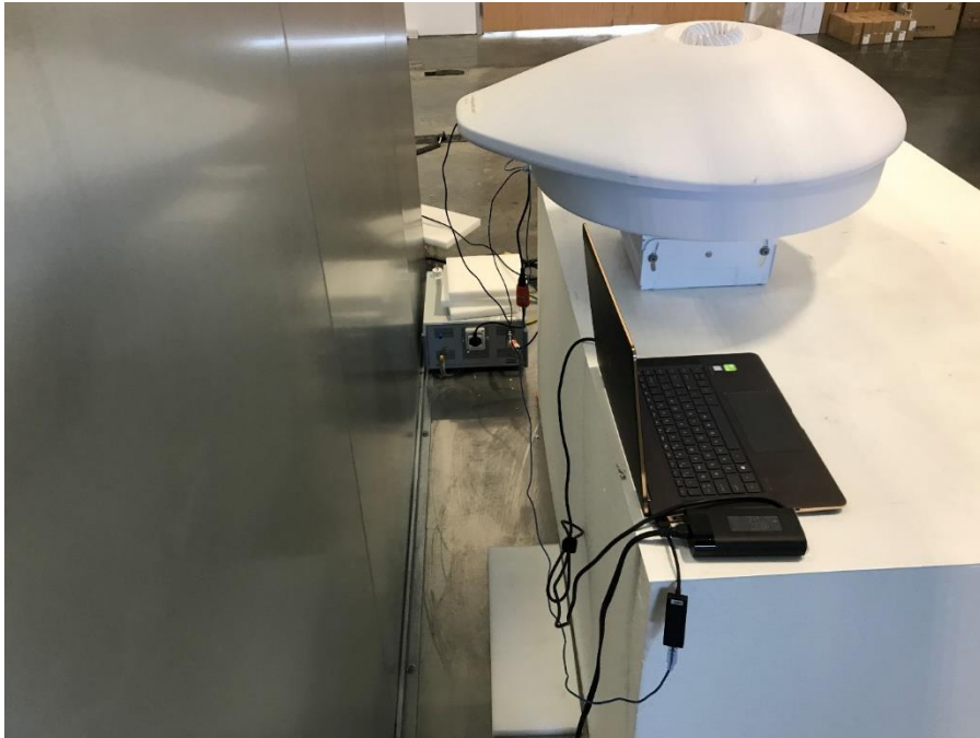
Photograph 5: Back View Test Set Up AC Mains Conducted Emissions
