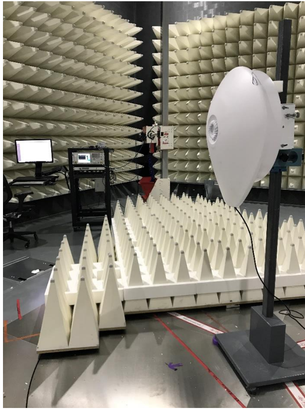
Photograph 3: View Test Set Up Radiated Emissions 17 - 40 GHz
