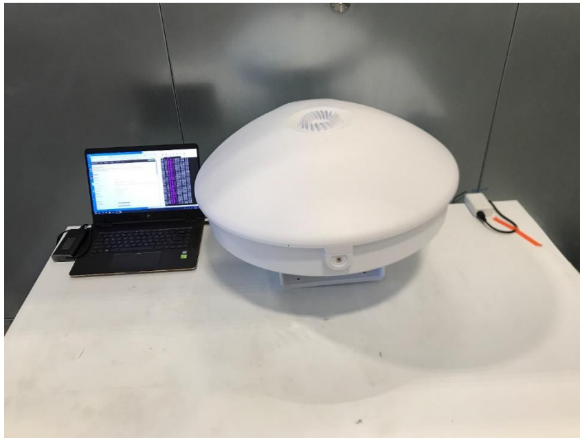
Photograph 4: Front View Test Set Up AC Mains Conducted Emissions
