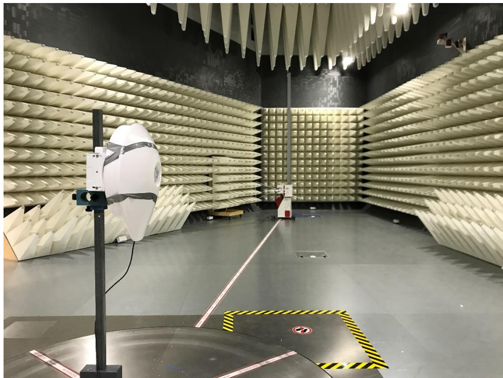
Photograph 1: Test Set Up Radiated Emissions 30 – 1000 MHz
