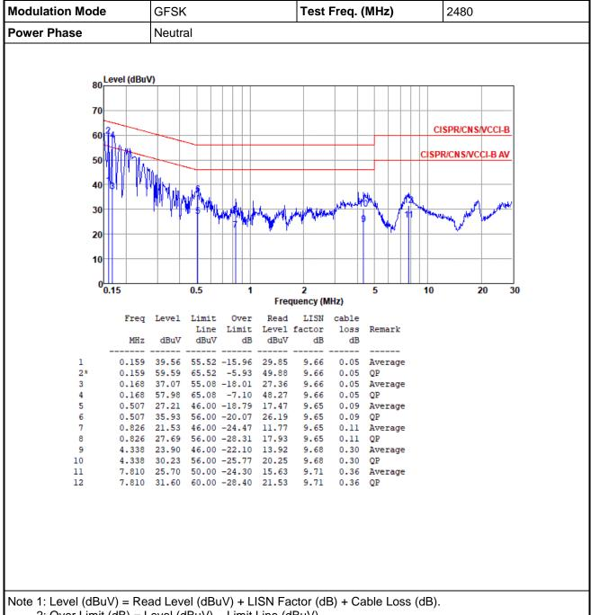
2: Over Limit (dB) = Level (dBuV) – Limit Line (dBuV).
