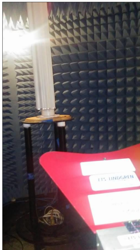
Photograph 4. Test Setup, Radiated Emissions Above 1GHz, 22dBi antenna
