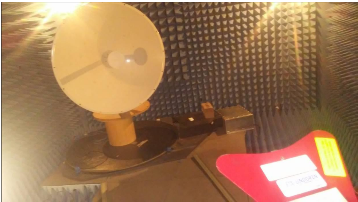
Photograph 2. Test Setup, Radiated Emissions Above 1GHz, 34dBi antenna
