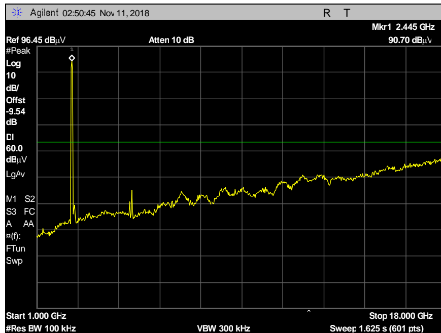
Plot 103. Conducted Spurious Emissions, Hopping, DH1, 1 GHz – 18 GHz
