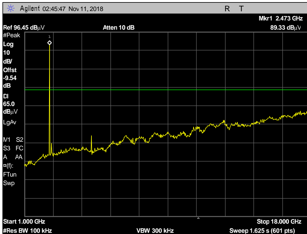
Plot 118. Conducted Spurious Emissions, Nonhopping, 2480MHz, 3-DH5, 1 GHz – 18 GHz
