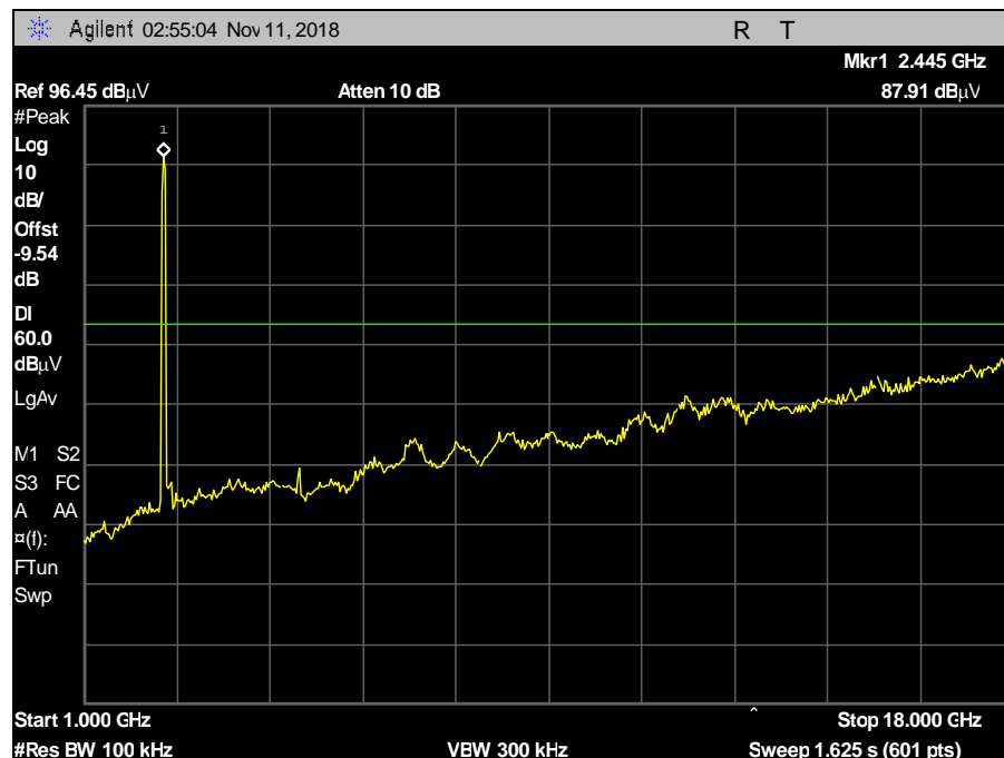
Plot 106. Conducted Spurious Emissions, Hopping, 3-DH5, 1 GHz – 18 GHz
