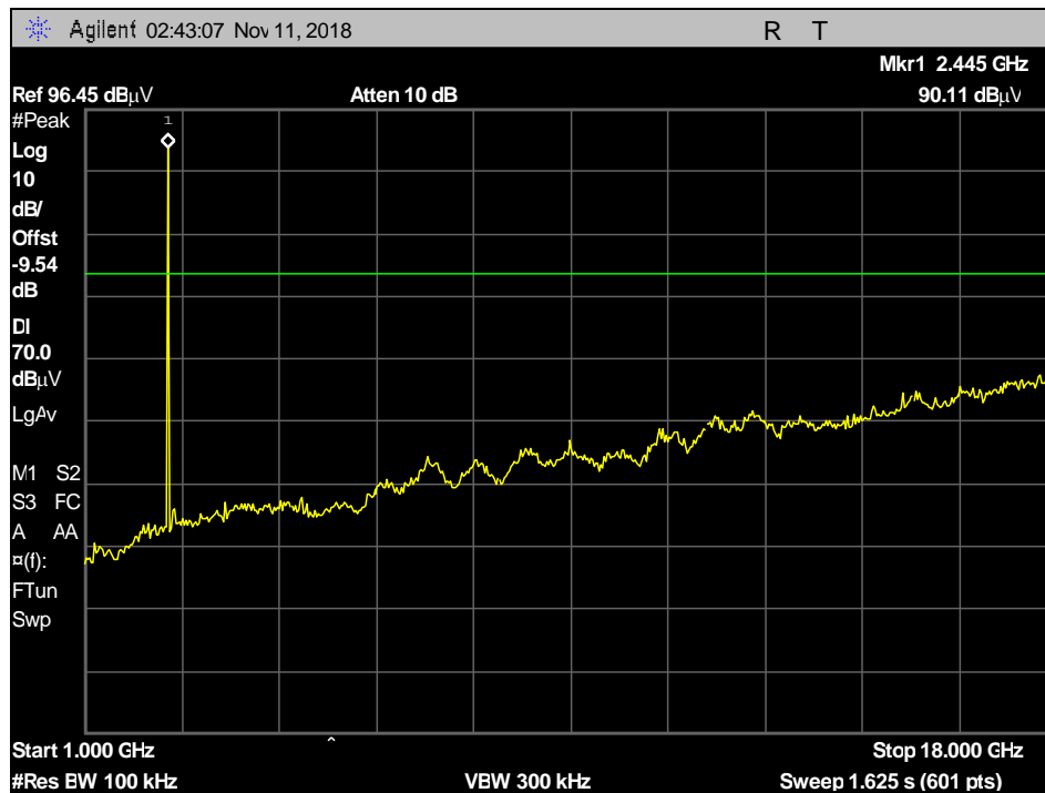
Plot 113. Conducted Spurious Emissions, Nonhopping, 2441MHz, 3-DH1, 1 GHz – 18 GHz
