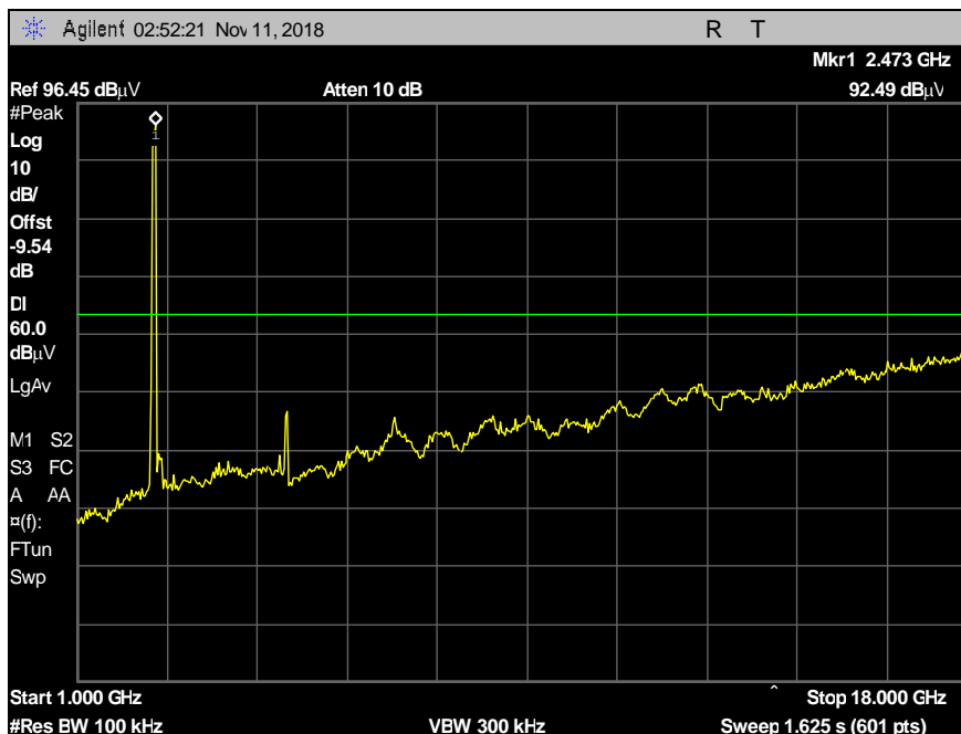
Plot 104. Conducted Spurious Emissions, Hopping, DH5, 1 GHz – 18 GHz
