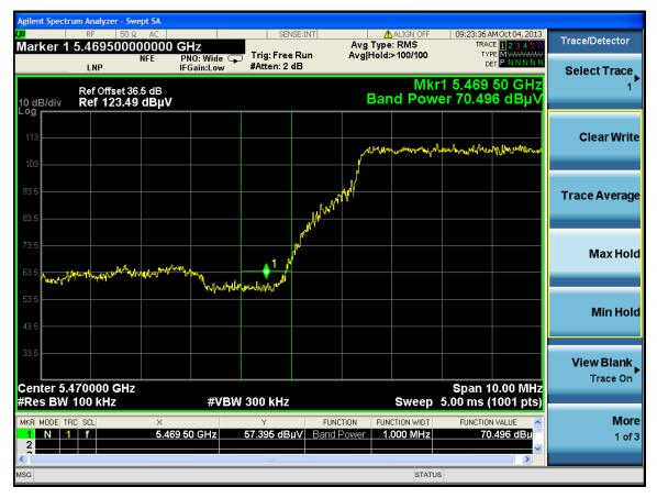
Standard Method > 2 MHz from band edge (1 MHz RBW, 3 MHz VBW)  $EIRP[dBm] = E[dB\mu V/m] + 20 \log(d[meters]) - 104.77$ Measurement:  $= 74.767 \text{ dB}\mu\text{V/m} + 20 \log(1 \text{ meter}) - 104.77$
