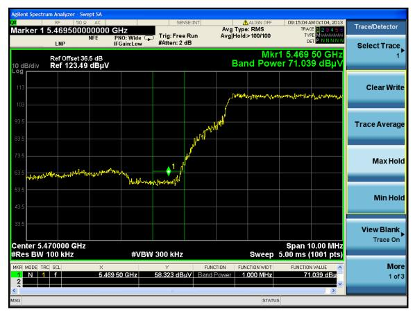
$\begin{array}{ll} Standard\ Method \geq 2\ MHz\ from\ band\ edge\ (1\ MHz\ RBW,\ 3\ MHz\ VBW) \\ Measurement: & EIRP[dBm] = E[dB\mu V/m] + 20\ log(d[meters]) - 104.77 \\ & = 74.915\ dB\mu V/m + 20\ log(1\ meter) - 104.77 \end{array}$
