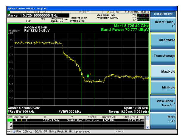
$\begin{array}{ll} Standard\ Method \geq 2\ MHz\ from\ band\ edge\ (1\ MHz\ RBW,\ 3\ MHz\ VBW) \\ Measurement: & EIRP[dBm] = E[dB\mu V/m] + 20\ log(d[meters]) - 104.77 \\ & = 75.479\ dB\mu V/m + 20\ log(1\ meter) - 104.77 \end{array}$
