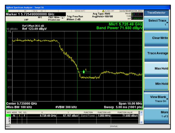
$\begin{array}{ll} Standard\ Method \geq 2\ MHz\ from\ band\ edge\ (1\ MHz\ RBW,\ 3\ MHz\ VBW) \\ Measurement: & EIRP[dBm] = E[dB\mu V/m] + 20\ log(d[meters]) - 104.77 \\ & = 75.227\ dB\mu V/m + 20\ log(1\ meter) - 104.77 \end{array}$
