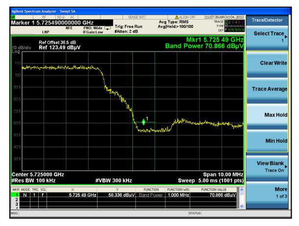
$\begin{array}{ll} Standard\ Method \geq 2\ MHz\ from\ band\ edge\ (1\ MHz\ RBW,\ 3\ MHz\ VBW) \\ Measurement: & EIRP[dBm] = E[dB\mu V/m] + 20\ log(d[meters]) - 104.77 \\ & = 75.545\ dB\mu V/m + 20\ log(1\ meter) - 104.77 \end{array}$
