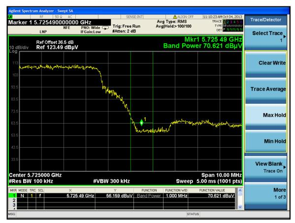
$\begin{array}{ll} Standard\ Method \geq 2\ MHz\ from\ band\ edge\ (1\ MHz\ RBW,\ 3\ MHz\ VBW) \\ Measurement: & EIRP[dBm] = E[dB\mu V/m] + 20\ log(d[meters]) - 104.77 \\ & = 75.505\ dB\mu V/m + 20\ log(1\ meter) - 104.77 \end{array}$
