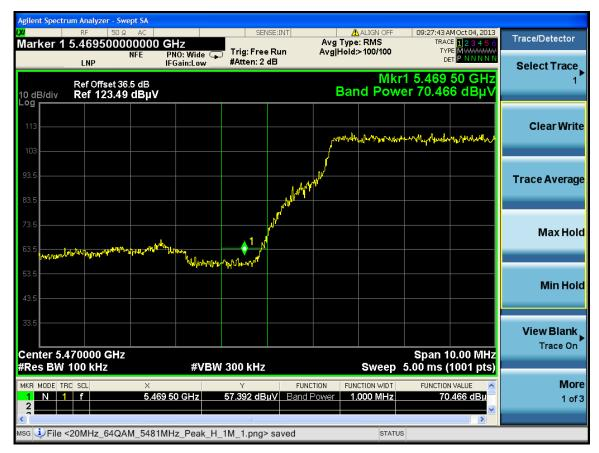
Standard Method > 2 MHz from band edge (1 MHz RBW, 3 MHz VBW) Measurement:  $EIRP[dBm] = E[dB\mu V/m] + 20 \ log(d[meters]) - 104.77 \\ = 75.024 \ dB\mu V/m + 20 \ log(1 \ meter) - 104.77$
