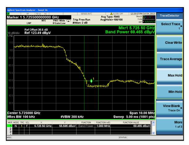
$\begin{array}{ll} Standard\ Method \geq 2\ MHz\ from\ band\ edge\ (1\ MHz\ RBW,\ 3\ MHz\ VBW) \\ Measurement: & EIRP[dBm] = E[dB\mu V/m] + 20\ log(d[meters]) - 104.77 \\ & = 73.880\ dB\mu V/m + 20\ log(1\ meter) - 104.77 \end{array}$
