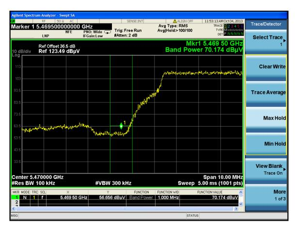
$\begin{array}{ll} Standard\ Method \geq 2\ MHz\ from\ band\ edge\ (1\ MHz\ RBW,\ 3\ MHz\ VBW) \\ Measurement: & EIRP[dBm] = E[dB\mu V/m] + 20\ log(d[meters]) - 104.77 \\ & = 74.369\ dB\mu V/m + 20\ log(1\ meter) - 104.77 \end{array}$
