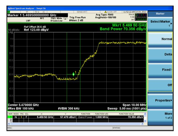
$\begin{array}{ll} Standard\ Method > 2\ MHz\ from\ band\ edge\ (1\ MHz\ RBW,\ 3\ MHz\ VBW) \\ Measurement: & EIRP[dBm] = E[dB\mu V/m] + 20\ log(d[meters]) - 104.77 \\ & = 74.092\ dB\mu V/m + 20\ log(1\ meter) - 104.77 \end{array}$
