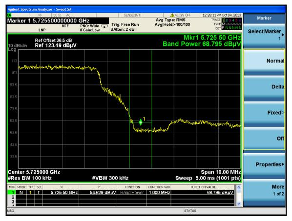
$\begin{array}{ll} Standard\ Method \geq 2\ MHz\ from\ band\ edge\ (1\ MHz\ RBW,\ 3\ MHz\ VBW) \\ Measurement: & EIRP[dBm] = E[dB\mu V/m] + 20\ log(d[meters]) - 104.77 \\ & = 73.512\ dB\mu V/m + 20\ log(1\ meter) - 104.77 \end{array}$
