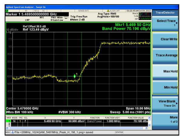
$\begin{array}{ll} Standard\ Method \geq 2\ MHz\ from\ band\ edge\ (1\ MHz\ RBW,\ 3\ MHz\ VBW) \\ Measurement: & EIRP[dBm] = E[dB\mu V/m] + 20\ log(d[meters]) - 104.77 \\ & = 75.033\ dB\mu V/m + 20\ log(1\ meter) - 104.77 \end{array}$
