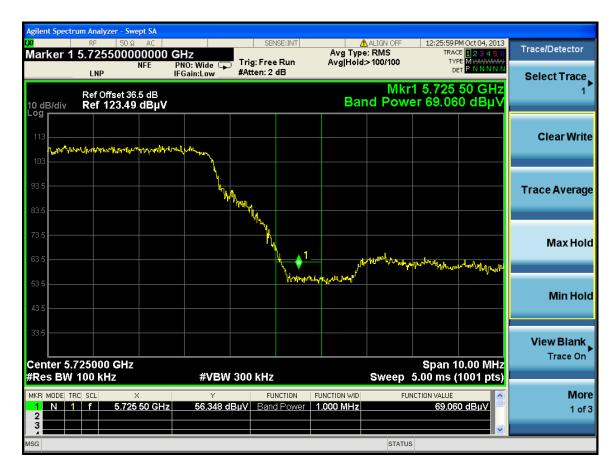
$\begin{array}{ll} Standard\ Method \geq 2\ MHz\ from\ band\ edge\ (1\ MHz\ RBW,\ 3\ MHz\ VBW) \\ Measurement: & EIRP[dBm] = E[dB\mu V/m] + 20\ log(d[meters]) - 104.77 \\ & = 73.466\ dB\mu V/m + 20\ log(1\ meter) - 104.77 \end{array}$
