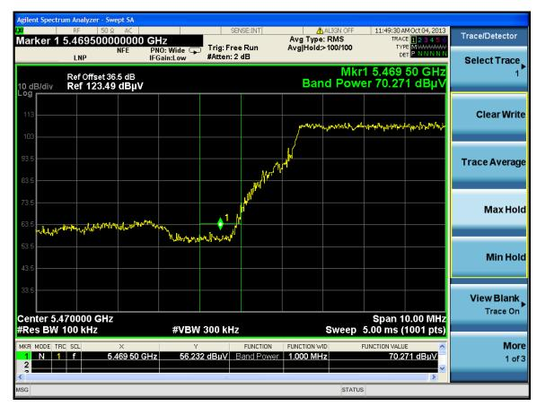
$\begin{array}{ll} Standard\ Method \geq 2\ MHz\ from\ band\ edge\ (1\ MHz\ RBW,\ 3\ MHz\ VBW) \\ Measurement: & EIRP[dBm] = E[dB\mu V/m] + 20\ log(d[meters]) - 104.77 \\ & = 74.327\ dB\mu V/m + 20\ log(1\ meter) - 104.77 \end{array}$
