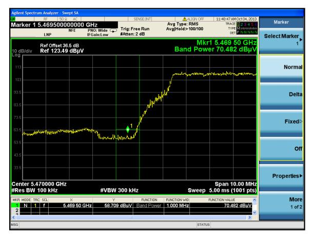
Standard Method > 2 MHz from band edge (1 MHz RBW, 3 MHz VBW) Measurement:  $EIRP[dBm] = E[dB\mu V/m] + 20 log(d[meters]) - 104.77 \\ = 74.075 dB\mu V/m + 20 log(1 meter) - 104.77 \\ = -30.69 dBm/MHz$
