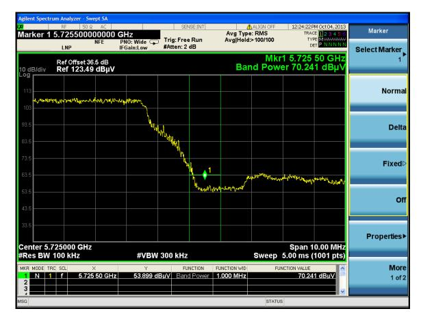
Standard Method > 2 MHz from band edge (1 MHz RBW, 3 MHz VBW) Measurement:  $EIRP[dBm] = E[dB\mu V/m] + 20 \ log(d[meters]) - 104.77 \\ = 73.464 \ dB\mu V/m + 20 \ log(1 \ meter) - 104.77 \\ = -31.30 \ dBm/MHz$
