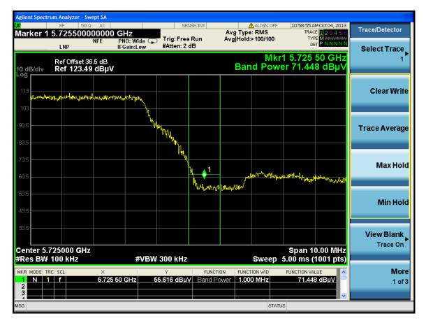
Standard Method > 2 MHz from band edge (1 MHz RBW, 3 MHz VBW) Measurement:  $EIRP[dBm] = E[dB\mu V/m] + 20 \ log(d[meters]) - 104.77 \\ = 75.452 \ dB\mu V/m + 20 \ log(1 \ meter) - 104.77$
