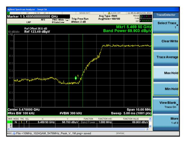
Standard Method > 2 MHz from band edge (1 MHz RBW, 3 MHz VBW) Measurement:  $EIRP[dBm] = E[dB\mu V/m] + 20 \log(d[meters]) - 104.77 \\ = 74.278 \ dB\mu V/m + 20 \log(1 \ meter) - 104.77 \\ = -30.49 \ dBm/MHz$
