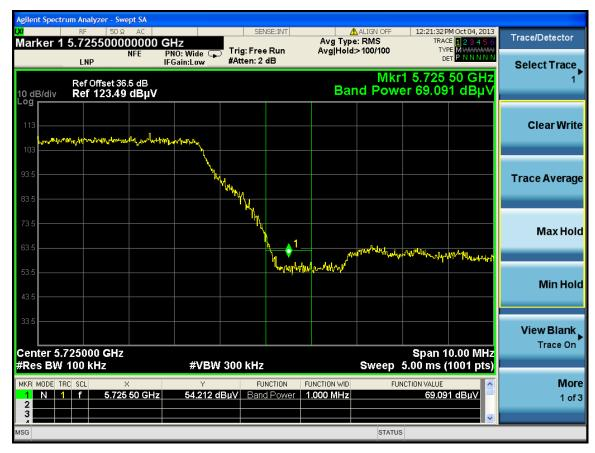
$\begin{array}{ll} Standard\ Method > 2\ MHz\ from\ band\ edge\ (1\ MHz\ RBW,\ 3\ MHz\ VBW) \\ Measurement: & EIRP[dBm] = E[dB\mu V/m] + 20\ log(d[meters]) - 104.77 \\ & = 73.352\ dB\mu V/m + 20\ log(1\ meter) - 104.77 \end{array}$
