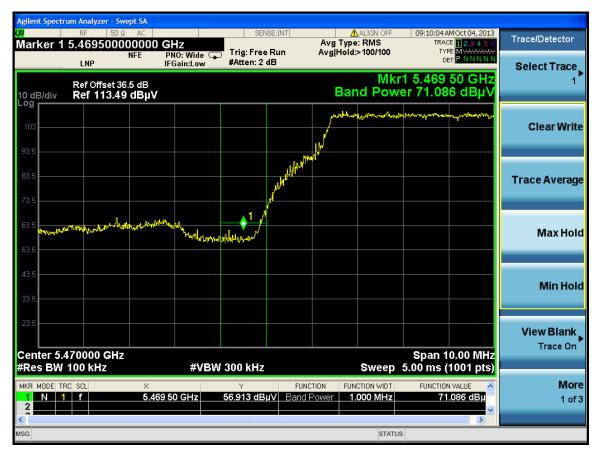
Standard Method > 2 MHz from band edge (1 MHz RBW, 3 MHz VBW) Measurement:  $EIRP[dBm] = E[dB\mu V/m] + 20 \log(d[meters]) - 104.77$  $= 74.778 \ dB\mu V/m + 20 \log(1 \ meter) - 104.77$
