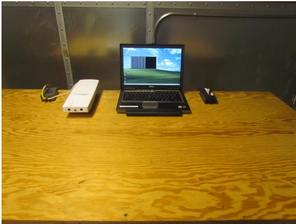
Conducted Emissions – PoE Powered Front View
