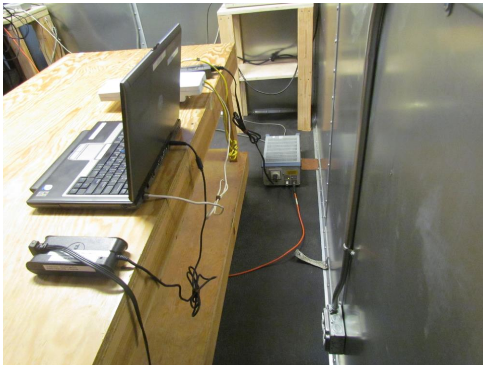
Conducted Emissions – PoE Powered Side View
