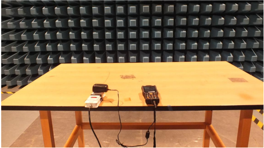
FCC Part 22H/24E Radiated Emission above 1GHz -Front
