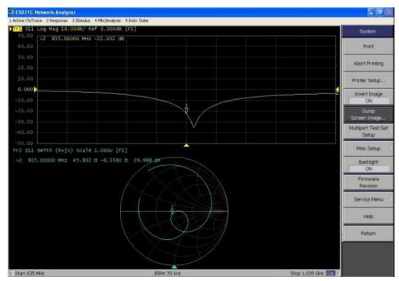
D835V2, serial No. 4d141 Extended Dipole Calibrations
