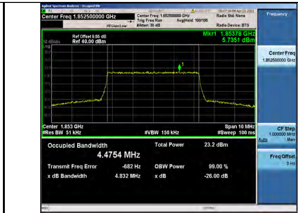
Band2-5MHz-16QAM-18625-25RB#0-4.4754
