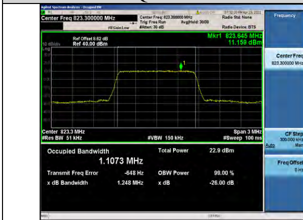
Band26-1.4MHz-QPSK-26783-6RB#0-1.1073
