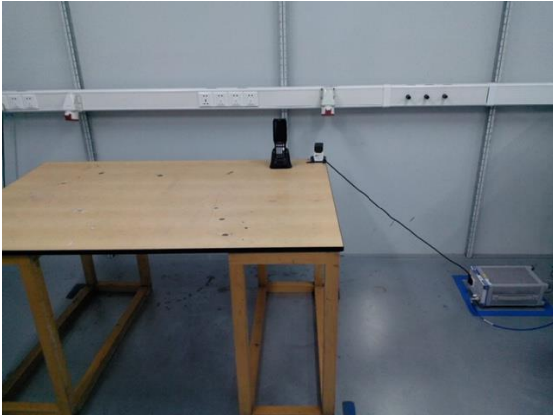
AC Conducted Emission Test Setup -Front
