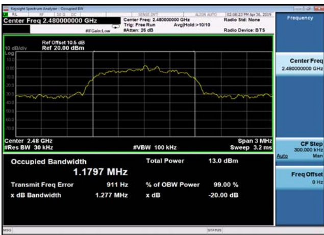
20dB Bandwidth: 8DPSK,2480MHz,3DH5
