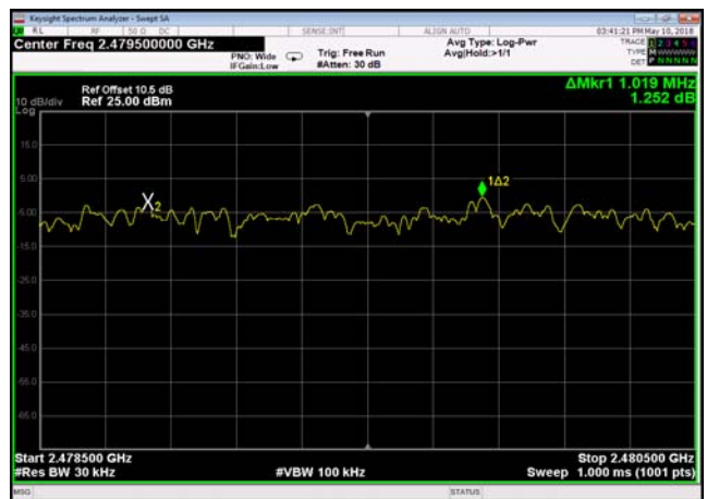
Carrier Frequency Separation: GFSK, Hopping DH5 2440.5~2442.5
