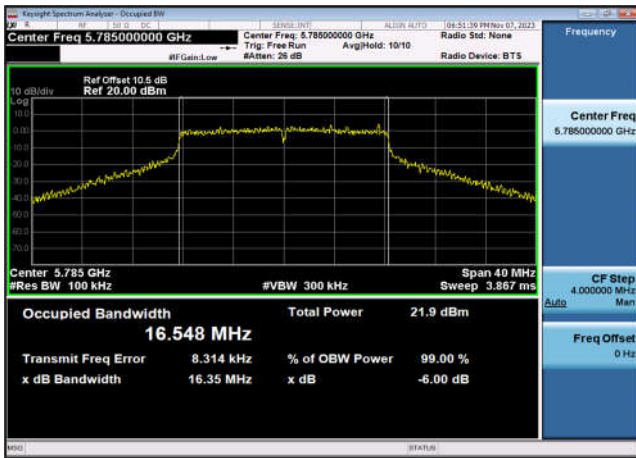
U-NII-3 6dB Bandwidth-802.11ac(20MHz) ,5745MHz,Ant1
