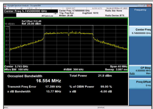
U-NII-3 6dB Bandwidth-802.11a(20MHz) ,5745MHz,Ant1
