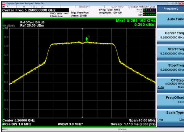
U-NII-2a Power spectral density-802.1 1ac(20MHz),5320MHz,Ant1
