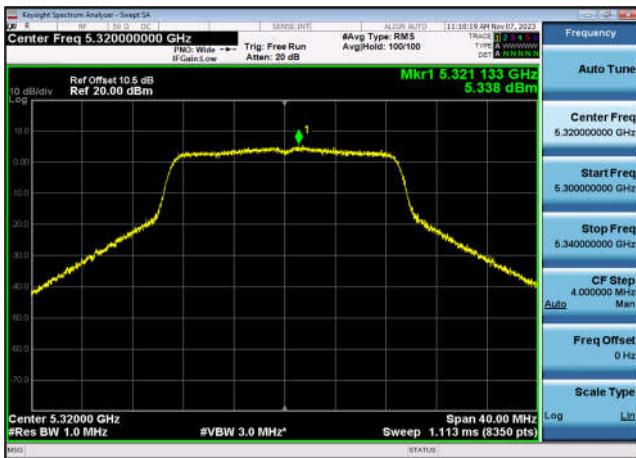
U-NII-2a Power spectral density-802.1 1ac(20MHz),5320MHz,Ant1
