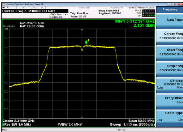
U-NII-2a Power spectral density-802.1 1n(40MHz),5310MHz,Ant1
