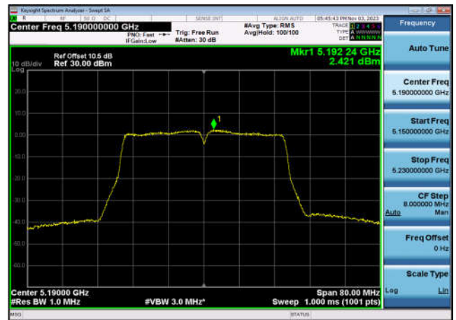
U-NII-1 Power spectral density-802.11 ac(40MHz),5190MHz,Ant1
