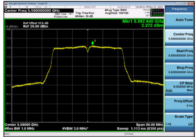
U-NII-2c Power spectral density-802.1 1ac(80MHz),5530MHz,Ant1
