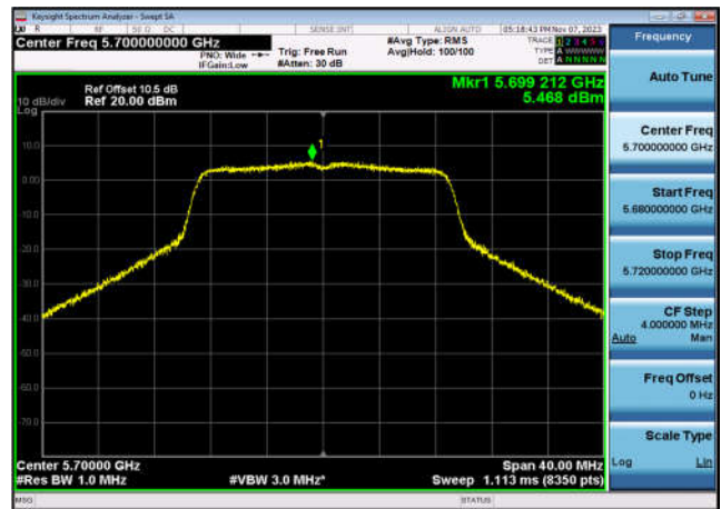
U-NII-2c Power spectral density-802.1 1ac(20MHz),5700MHz,Ant1
