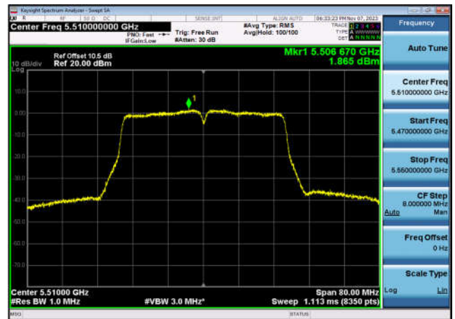
U-NII-2c Power spectral density-802.1 1n(40MHz),5670MHz,Ant1
