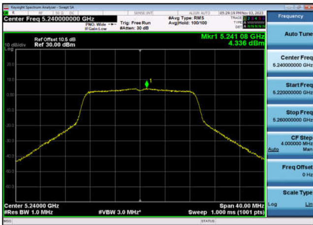
U-NII-1 Power spectral density-802.11 ac(20MHz),5240MHz,Ant1
