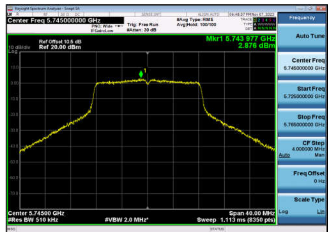
U-NII-3 Power spectral density-802.11 a(20MHz),5745MHz,Ant1
