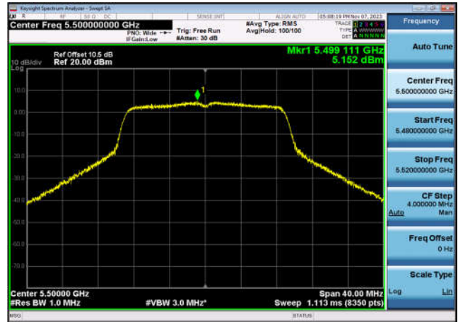
U-NII-2c Power spectral density-802.1 1ac(20MHz),5700MHz,Ant1
