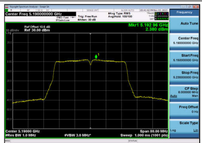
U-NII-1 Power spectral density-802.11 a(20MHz),5180MHz,Ant1
