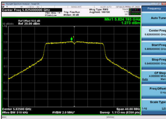
U-NII-3 Power spectral density-802.11 n(40MHz),5795MHz,Ant1
