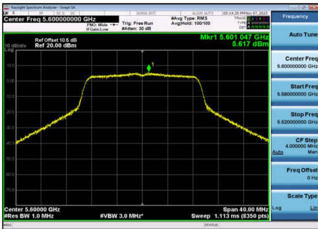
U-NII-2c Power spectral density-802.1 1ac(20MHz),5600MHz,Ant1
