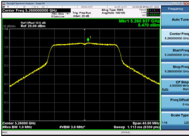
U-NII-2a Power spectral density-802.1 1n(20MHz),5320MHz,Ant1
