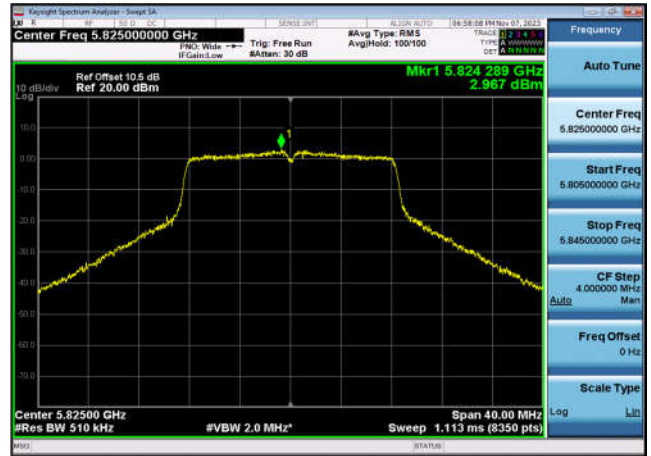
U-NII-3 Power spectral density-802.11 ac(20MHz),5785MHz,Ant1
