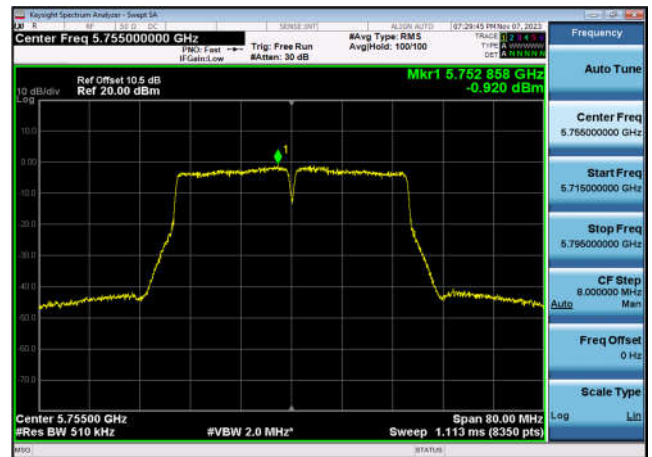
U-NII-3 Power spectral density-802.11 a(20MHz),5745MHz,Ant1
