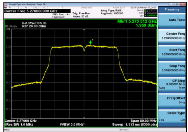
U-NII-2a Power spectral density-802.1 1ac(40MHz),5270MHz,Ant1
