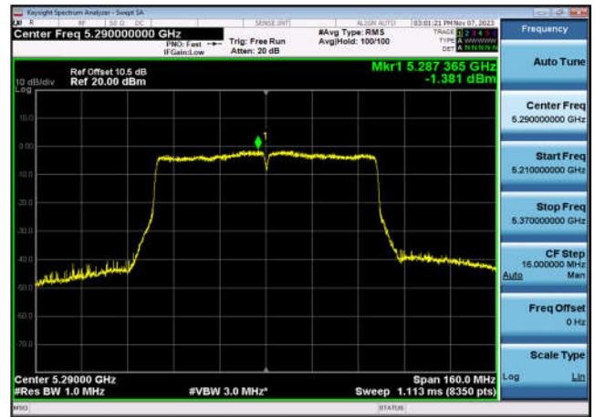
U-NII-2a Power spectral density-802.1 1ac(80MHz),5290MHz,Ant1
