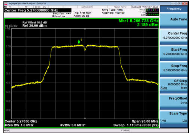
U-NII-2a Power spectral density-802.1 1a(20MHz),5260MHz,Ant1
