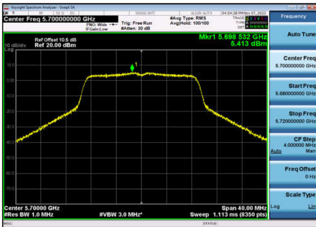
U-NII-2c Power spectral density-802.1 1n(40MHz),5590MHz,Ant1
