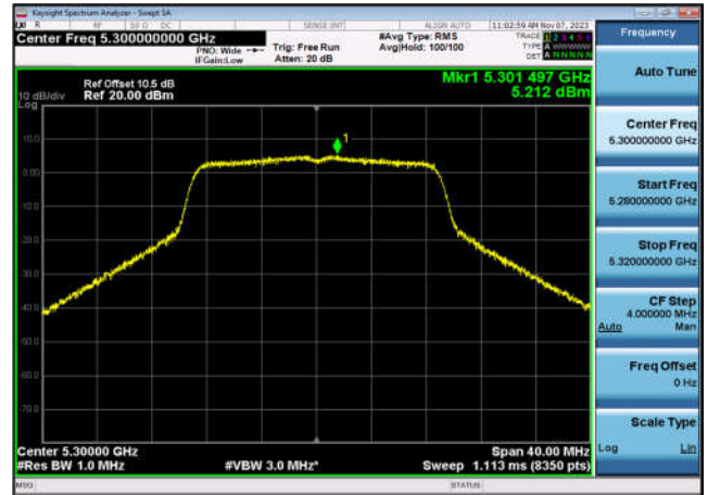
U-NII-2a Power spectral density-802.1 1ac(40MHz),5270MHz,Ant1
