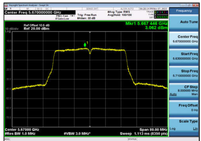
U-NII-2c Power spectral density-802.1 1n(40MHz),5670MHz,Ant1
