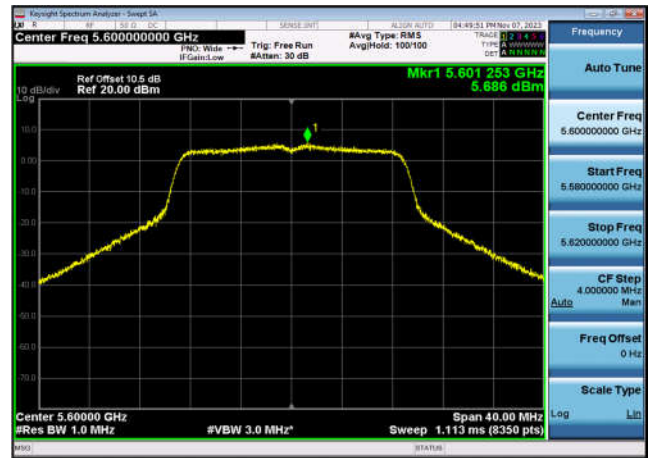
U-NII-2c Power spectral density-802.1 1n(40MHz),5510MHz,Ant1
