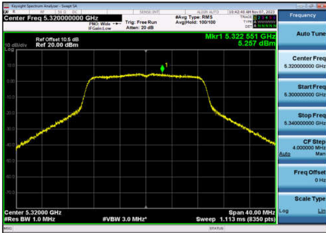
U-NII-2a Power spectral density-802.1 1n(40MHz),5310MHz,Ant1
