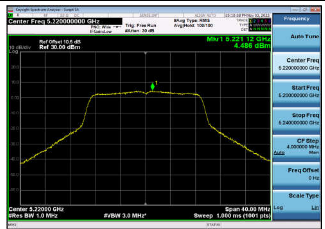
U-NII-1 Power spectral density-802.11 n(40MHz),5190MHz,Ant1
