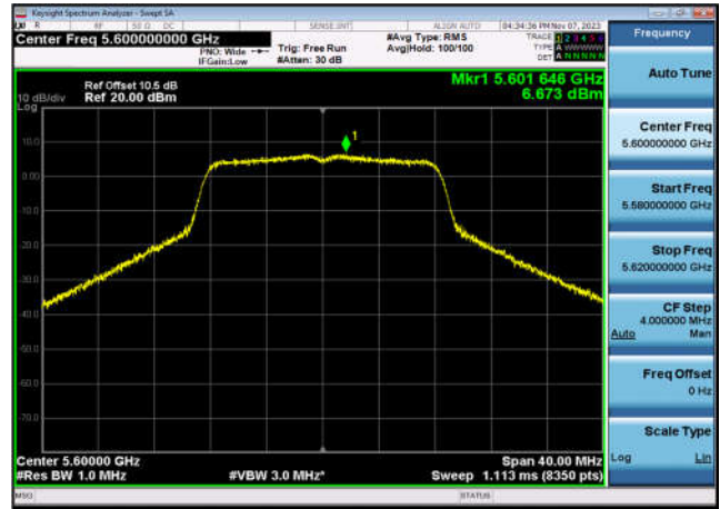
U-NII-2c Power spectral density-802.1 1ac(20MHz),5500MHz,Ant1
