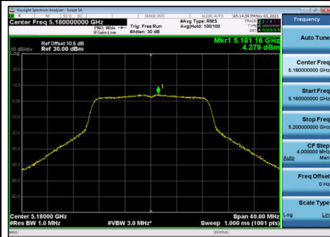
U-NII-1 Power spectral density-802.11 n(20MHz),5240MHz,Ant1
