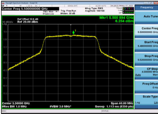
U-NII-2c Power spectral density-802.1 1a(20MHz),5700MHz,Ant1
