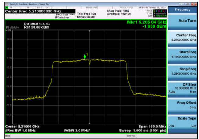
U-NII-1 Power spectral density-802.11 ac(80MHz),5210MHz,Ant1
