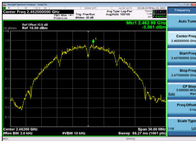
Power spectral density-802.11g ,2437MHz,Ant0
