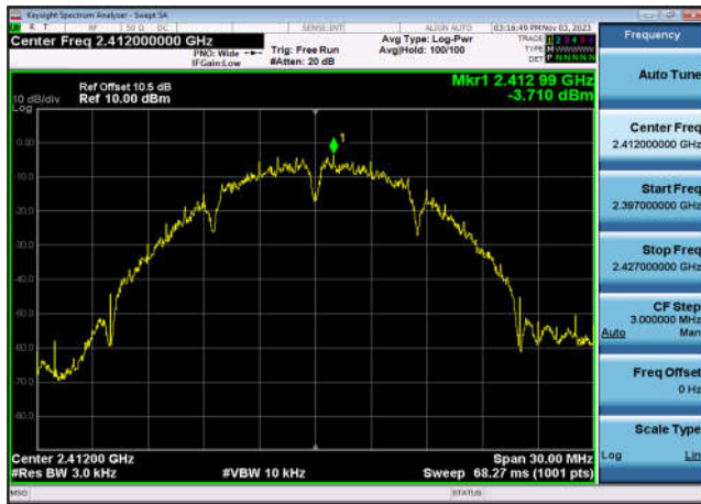
Power spectral density-802.11b ,2462MHz,Ant0
