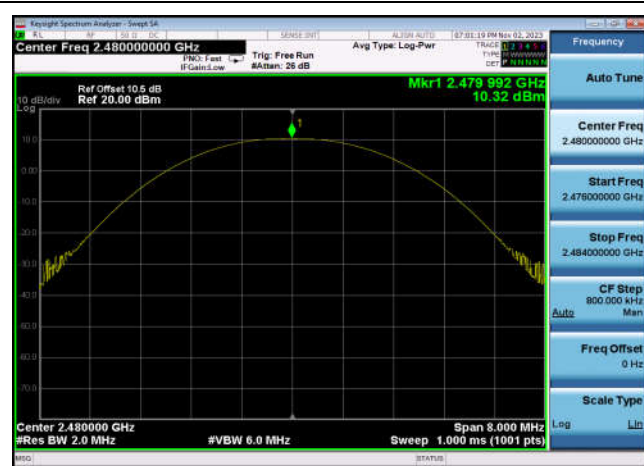
Output Power: DQPSK,2441MHz,2DH5
