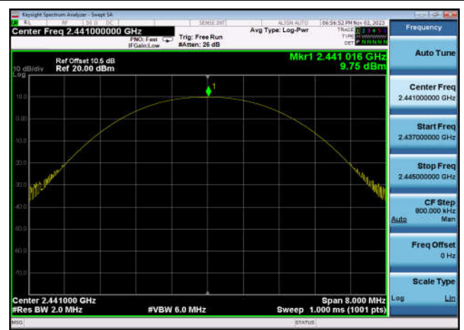
Output Power: DQPSK,2402MHz,2DH5
