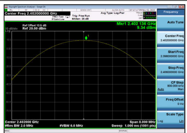
Output Power: DQPSK,2480MHz,2DH5
