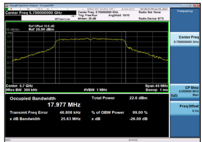
U-NII-2c 26dB&99% Bandwidth-802.11ac(40MHz),5590MHz,Ant1
