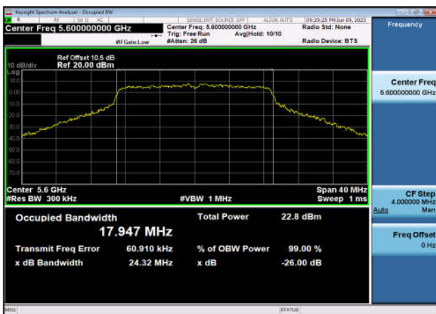
U-NII-2c 26dB&99% Bandwidth-802.11ac(40MHz),5510MHz,Ant1
