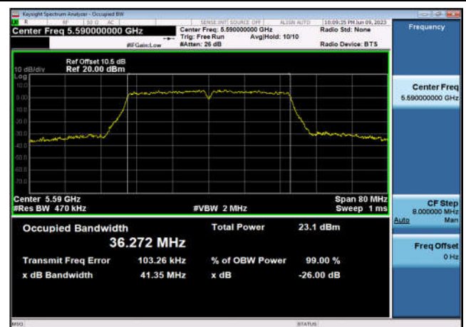
U-NII-2c 26dB&99% Bandwidth-802.11ac(40MHz),5590MHz,Ant1
