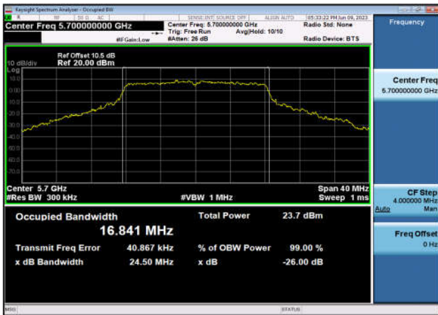
U-NII-2c 26dB&99% Bandwidth-802.11ac(20MHz),5600MHz,Ant1
