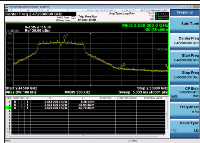
,Plot 2,Band Edge-802.11g,2462MHz ,Ant0
