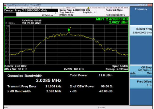
99% Bandwidth: 2480MHz – 2MHz bandwidth
