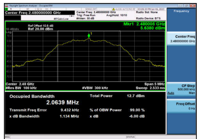
6dB Bandwidth: 2480MHz – 2MHz bandwidth
