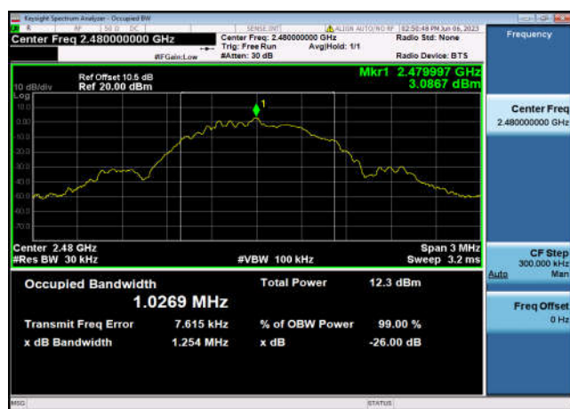
99% Bandwidth: 2480MHz – 1MHz bandwidth
