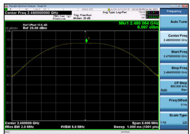
Output Power: 2480MHz – 2MHz bandwidth
