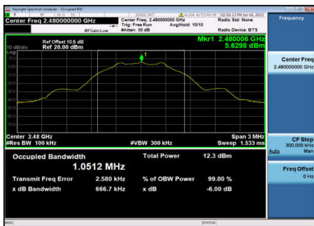
6dB Bandwidth: 2480MHz – 1MHz bandwidth
