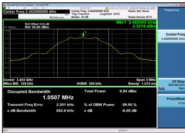
6dB Bandwidth: 2440MHz – 1MHz bandwidth
