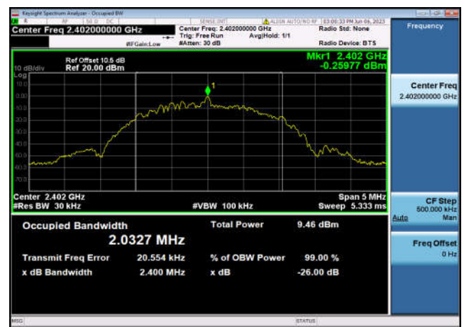
99% Bandwidth: 2440MHz – 2MHz bandwidth
