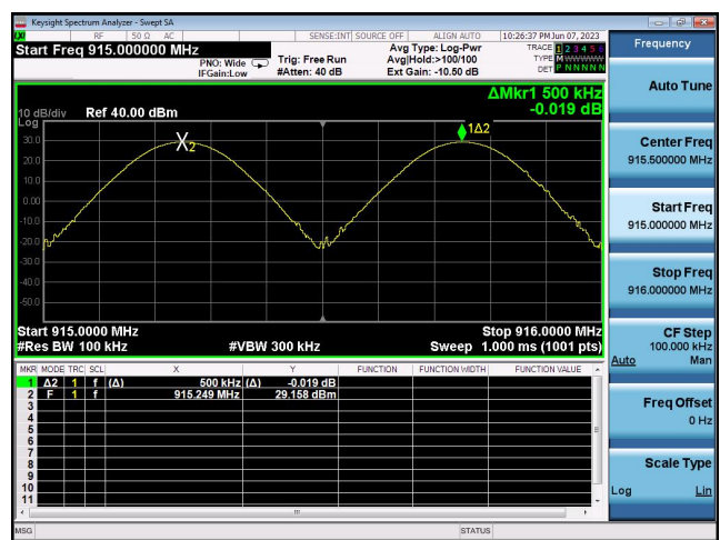
Carried Frequency Separation: 915.1~915.5MHz
