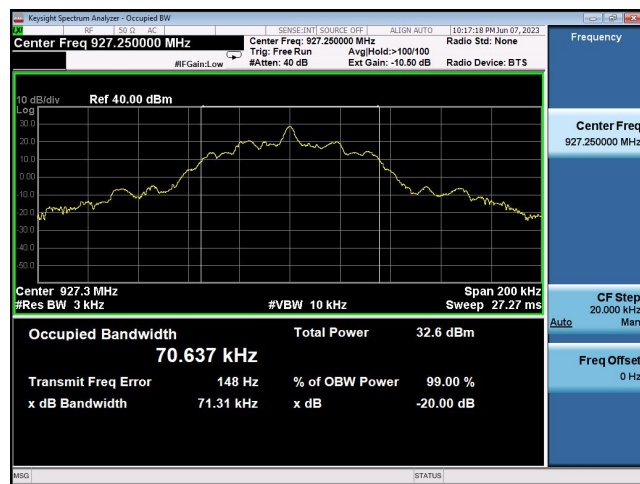
20dB Emission Bandwidth: 927.25MHz
