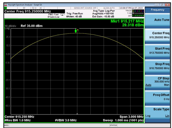
Conducted Output Power: 915.25MHz
