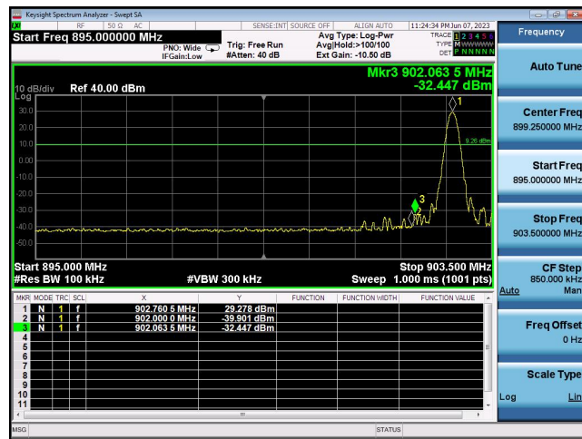
Conducted Band Edge: 902.75MHz_Hopping
