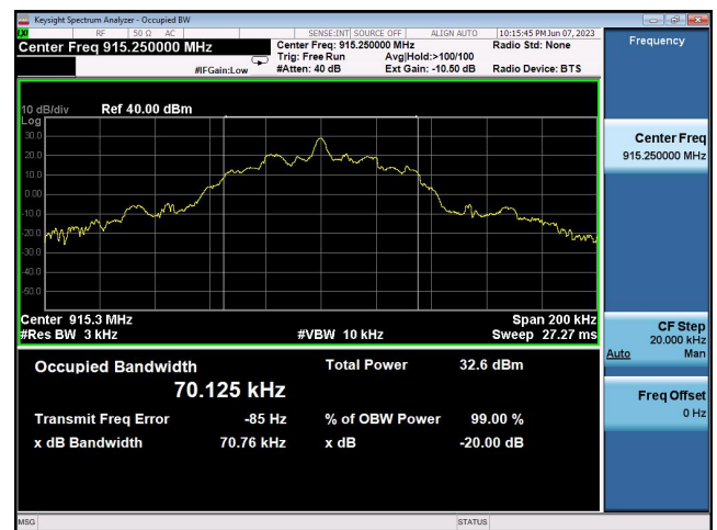
20dB Emission Bandwidth: 915.25MHz
