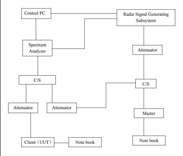
The UUT is a UNII device operating in client mode without radar detection. The radar test signals are injected into the master device.
