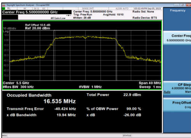
U-NII-2c 26dB&99% Bandwidth-802.11a(20MHz) ,5500MHz,Ant1
