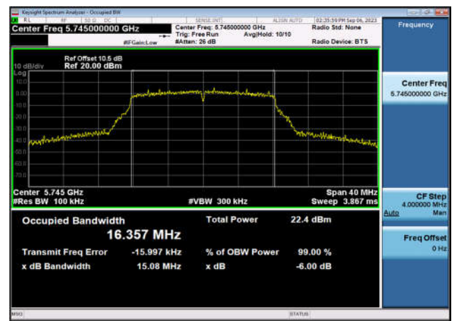
U-NII-3 6dB Bandwidth-802.11a(20MHz) ,5745MHz,Ant1
