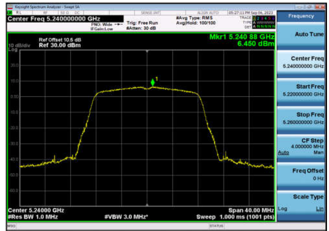
U-NII-1 Power spectral density-802.11 ac(20MHz),5220MHz,Ant1
