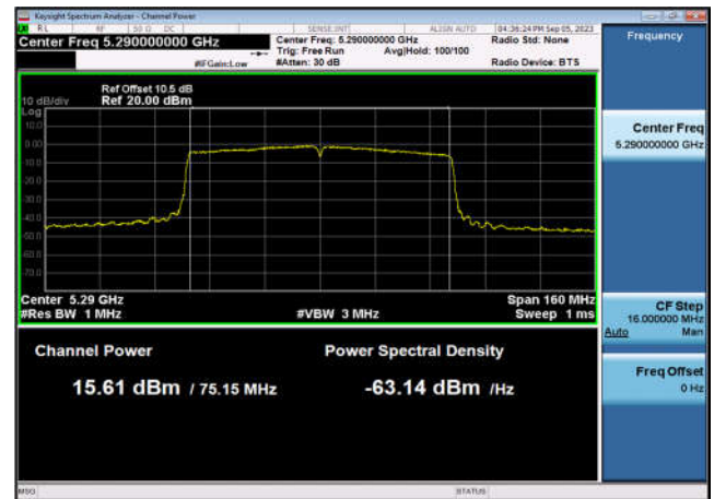
U-NII-2c Output Power-802.11n(20MHz) ,5600MHz,Ant1
