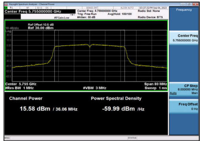
U-NII-3 Output Power-802.11a(20MHz) ,5745MHz,Ant1
