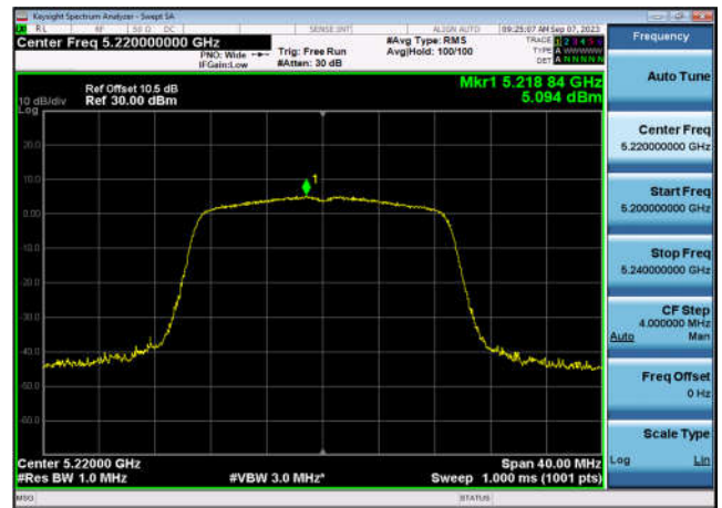
U-NII-1 Power spectral density-802.11 ac(40MHz),5190MHz,Ant1
