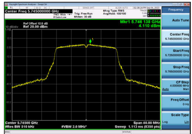
U-NII-3 Power spectral density-802.11 a(20MHz),5825MHz,Ant1
