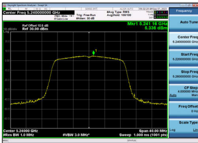
U-NII-1 Power spectral density-802.11 ac(20MHz),5240MHz,Ant1
