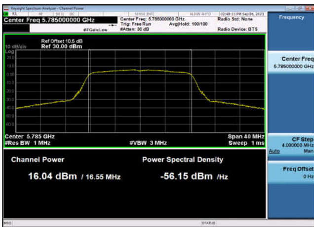
U-NII-3 Output Power-802.11a(20MHz) ,5785MHz,Ant1
