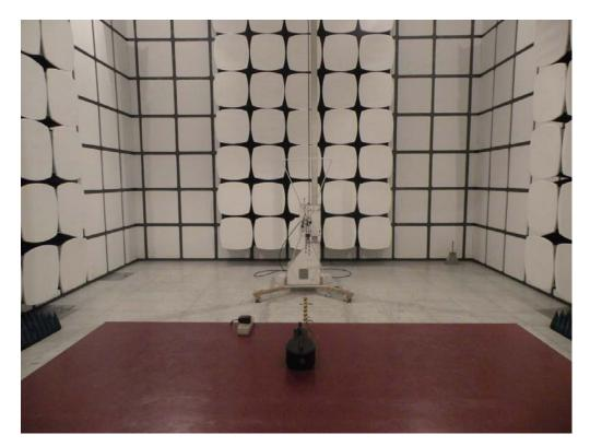
Radiated Emission Test Setup in Chamber
