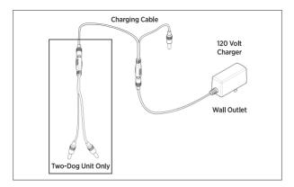
The Dogtra 280C uses a lithium polymer battery. Recharge the unit if the indicator light is red or does not come on, the transmitter LCD shows only 1 bar on the indicator, or the system will not stay on when any button is pressed.
