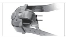
2. Press the charger onto the receiver until you hear a snap to secure the placement.
