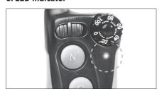
The LED indicator flashes every 4 seconds when the receiver is on and ready for use. The LED indicator will light up on both the transmitter and the receiver when the transmitter buttons are pressed.
