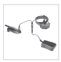
The Dogtra iQ MINI uses a lithium polymer battery. Recharge the unit if the indicator light is red or does not come on, or the system will not stay on when any button is pressed.
