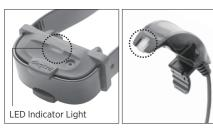
1. Align the clear plastic piece on the charger to the LED screen on the receiver.
