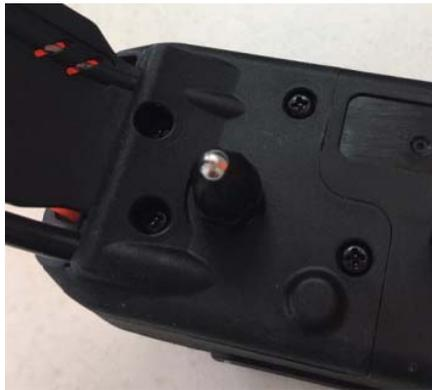
1.5.2 To maximize the signal with the GPS Collar, hold the GPS Connector with antenna facing up.
