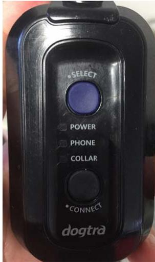
**Power** :The power LED blinks every 2 seconds while turned on. The LED color represents the battery life, with green (~50%), orange (~10%), and red (~0%). While charging and turned on, the LED will blink green.
