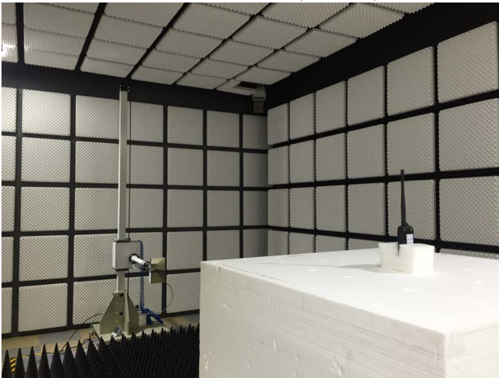
Radiated RF measurement (Above 1 GHz)
