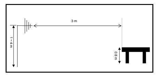
Radiated emission setup, above 1 GHz
