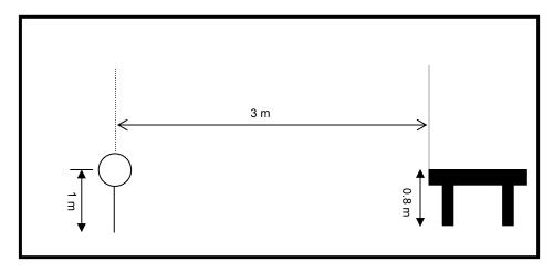
Radiated emission setup, below 1 000 MHz
